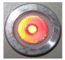
status; when the status indicator lamp shows red, it indicates that the program is setting status. (tips: if the lamp changes from green to red when the machine is in running status, press F5 into the running status again).
