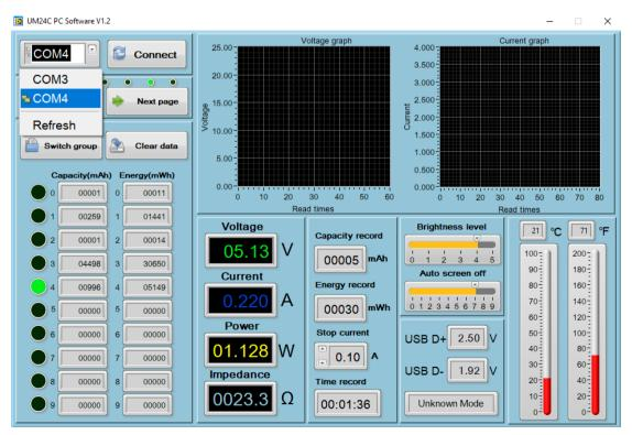
3.2.2 When the Bluetooth indicator changes from blinking to static, click "Connect"
