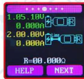
Data Connection Cable Impedance Measurement Interface
