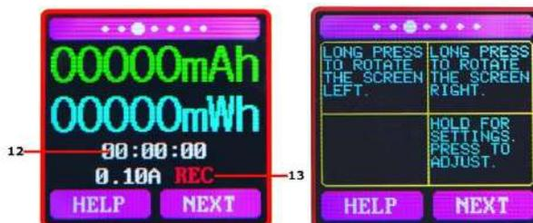
After power on, when the current flowing is greater than the Low Current trigger value. The system automatically begins to record the accumulated capacity, energy, and time elapsed. The 'REC' indicator will change from red to green.
