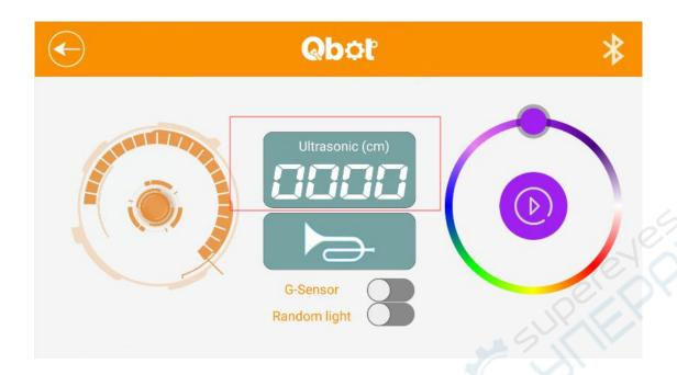
Then, you can click the Gravity control icon, and you can control the motion of Qbot by shaking your mobile phone. We offer two modes to control the motion of Qbot, and the other is stick mode, which means you can operate the Qbot through the virtual button on your phone.
