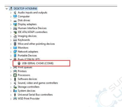
If you cannot find the corresponding USB port in the device manager, you need to install the driver again.
