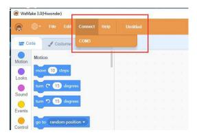
After clicking the corresponding serial port, the serial port connection is successful.
