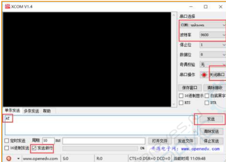
Figure 3: Send AT Command Diagram
