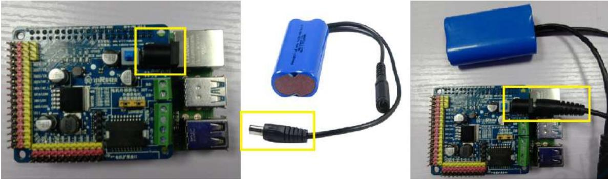
2、 Press the blue power switch button, the blue LED on the driver board lights up, wait about 30 seconds, if you see blue LEDs is flashing alternately, the system has started successfully.
