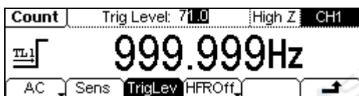
Figure 2-66 To set the high frequency on/off
