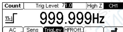
Figure 2-65 To set the trig level
