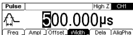
Figure 2-13 Pulse Signal Parameter Setting Interface
