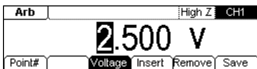
Figure 2-29 To Set the voltage
