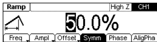
Figure 2-10 Ramp Signal Parameter Setting Interface
