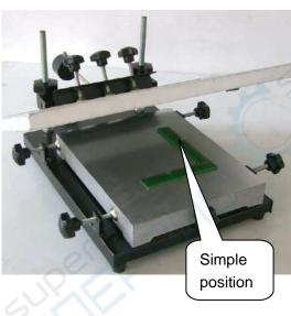
2. Make a simple position on the printer plate, place PCB and adjust handwheels to align stencil with PCB.
