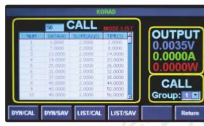
The spreadsheet embedded in the LCD , easy to do the output sequences and data settings
