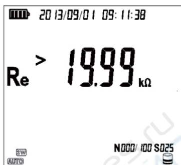
Earth resistance beyond measuring range
