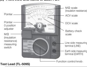
Removable test pin covers When not covered: CAT. II 1000 V When not covered Removable When attached : CAT Ⅲ 600 V Red Measuring cords Pin-type adapter Barriers Test pins Black CAT. III 600 V
