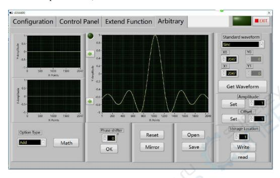
(4) keep the location choice, this series of machine with 0-15 waveform save location, select position 1 here, and then click on "write"; Blue bar said written progress;
