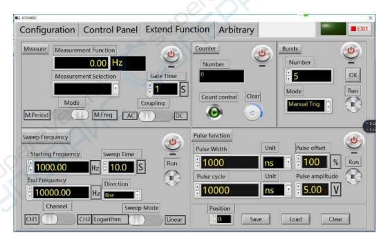
(3) connect the upper machine, switch to expand page, can control the output arbitrary waveform,
