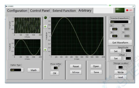
(4) Select operation type product, and then click operation button, generates the amplitude modulationwaveform.
