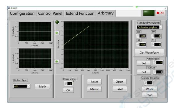
(5) In setting up starting point, end points, 800, 1601; Starting magnitude 8, termination of magnitude 8, then click the generated waveform, generated waveform is as follows:
