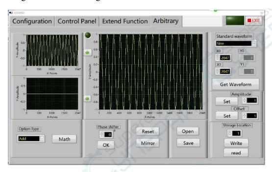
(3) Set the starting point 0; End point 2048, and then click "generate the waveform" button. Click the green arrow to the right generated waveform as shown:
