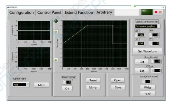
(6) In setting up starting point, end points, 1602, 2047; Starting magnitude 8, termination by 0, and then click the generated waveform, forming waveform as shown:
