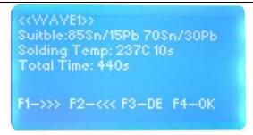
Press the "F4" button to return previous page. Press the temperature wave that the "F1" key carries out to make selection automatically, the process will shut down automatically upon completion and a warning buzzer will sound.
