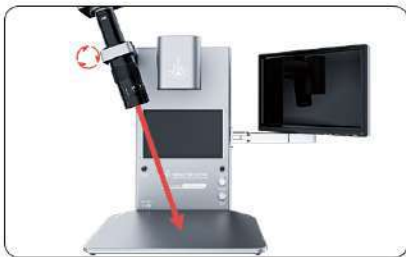
(1)调整显微镜镜头对准工作台 Align the microscope lens with the workbench
