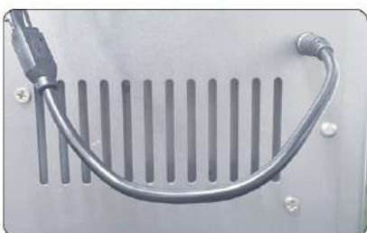
(1)DC线主接头连接机身接口 The main connector of DC line is connected to the rear interface of the fuselage
