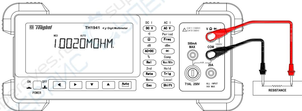
**Note:** Source current flows from the  $V\Omega$  to COM terminals
