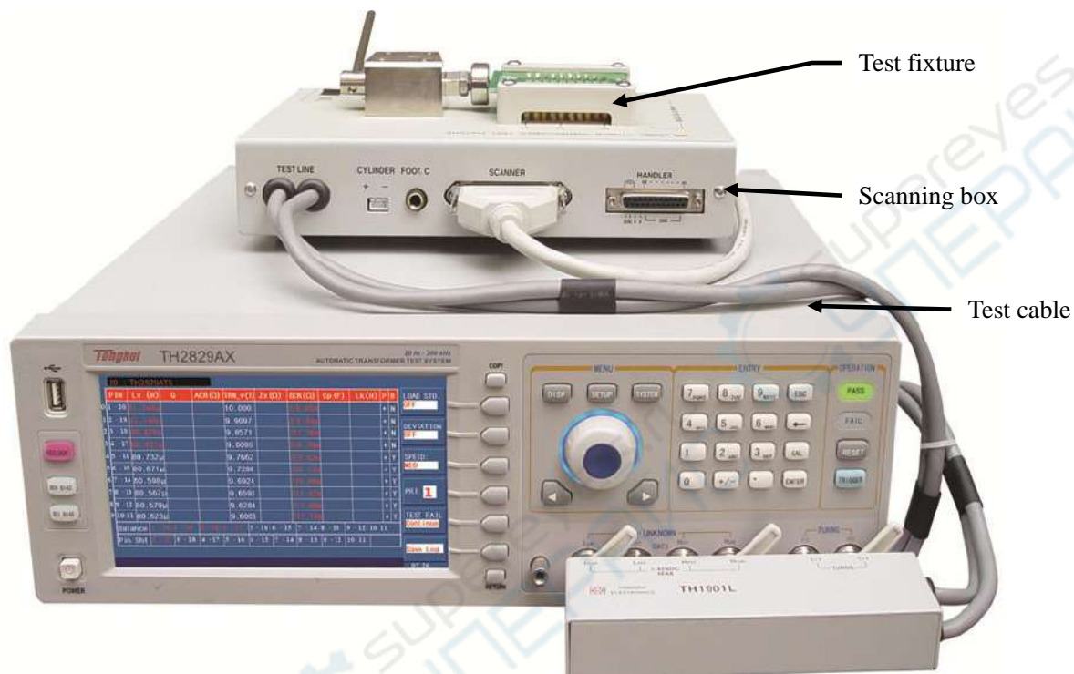
TH2829x702---Connect the scanning test cable to TH2829X
