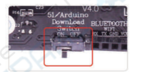
Put the switch to (OFF).
