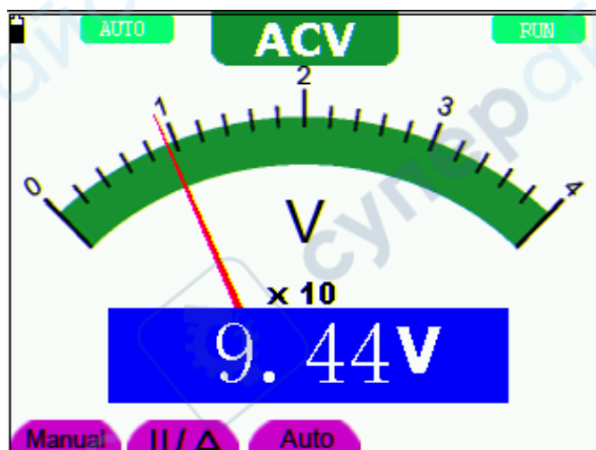
Figure 23: AC Voltage Measurement
