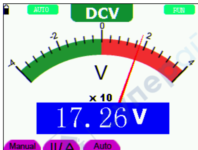
Figure 22: DC Voltage Measurement
