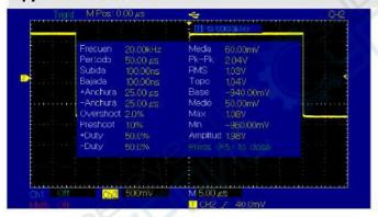
Multiple automatic parameter measurements
