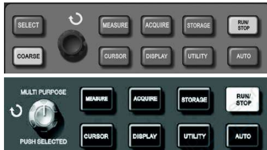
Figure 2-28 Function key (automatic measurement) of sampling system
