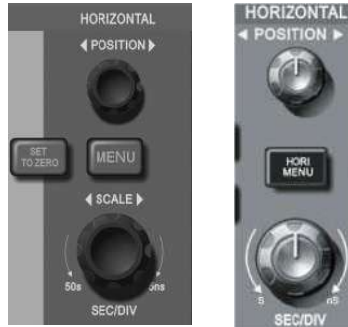
Figure 2-11 Interface of horizontal system
