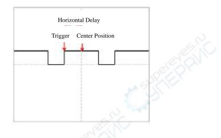
Figure 6-7 Horizontal Delay
