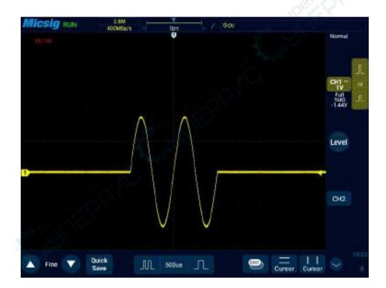
Figure 11-11 Segmented memory waveform acquisition
