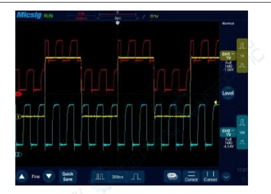
Figure 9-2 Mathematical Operation of CH1 adding CH2
