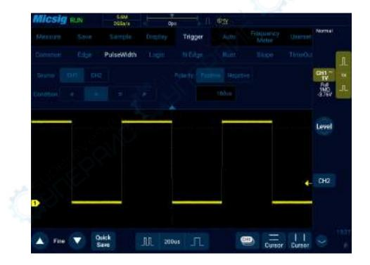
Figure 6-13 Pulse Width Trigger Setting Menu
