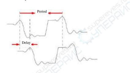
Figure 7-6 Phase Measurement Schematics
