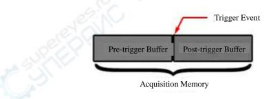
Figure 6-6 Conceptual Demonstration of Acquisition Memory
