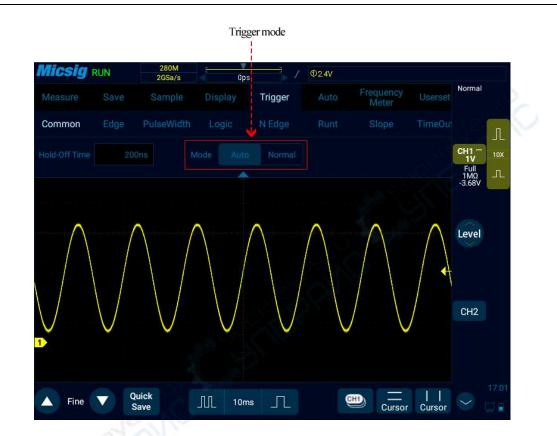
Figure 6-5 Oscilloscope Trigger Mode Setting
