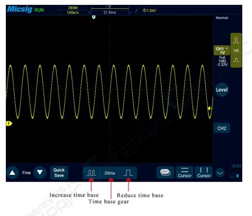
Figure 4-3 Adjust the Horizontal Time Base
