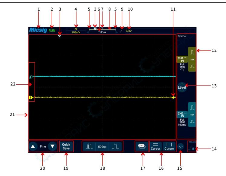
Figure 2-5 Oscilloscope Interface Display
