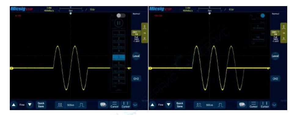
Figure 11-15 View after segment collection is completed
