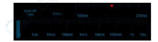
Figure 6-10 Trigger Hold-Off Time Set Interface
