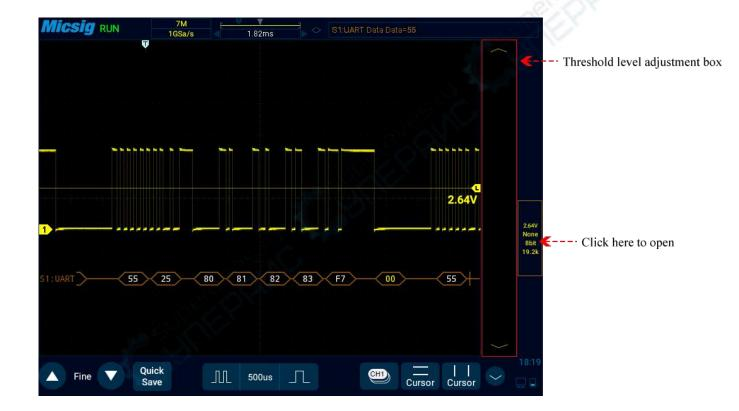
Figure 12-7 UART Decode Level Adjustment
