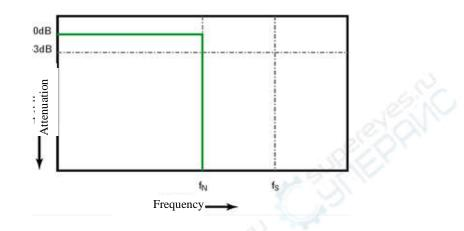
Figure 11-2 Theoretical Brick-Wall Frequency Response
