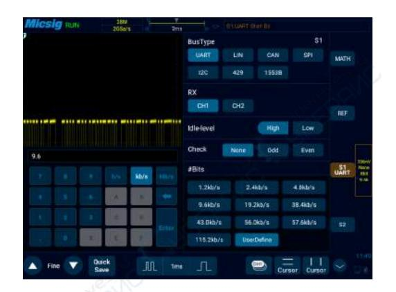
Figure 12-5 Baud Rate Default Setting
