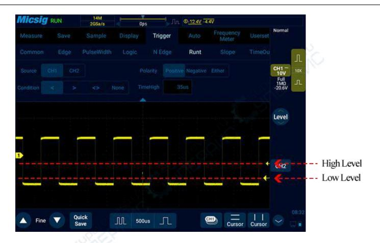
Figure 6-24 Runt Trigger Setting Menu
