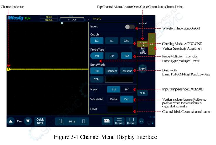
The ground level of each displayed analog channel signal is indicated by the channel indicator icon  $\square$  on the far left of the display screen.
