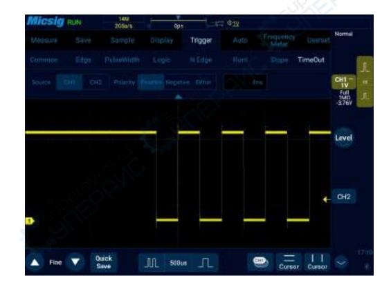
Figure 6-28 Time-out Trigger
