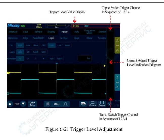
Trigger pulse width time can be set as 8ns~10s.
