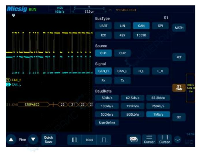
Figure 12-14 CAN Bus Configuration Menu
