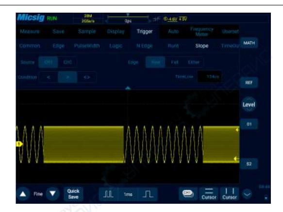
Figure 6-26 Slope Trigger Setting Menu
