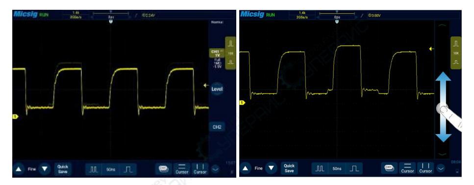
Figure 6-3 Abnormal Signal in Periodic Signals
