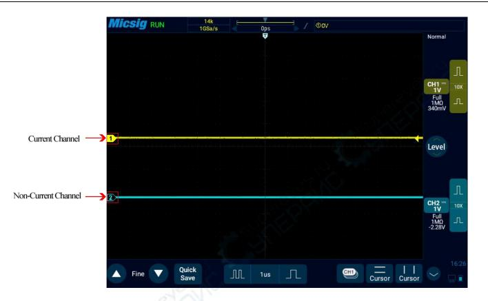
Figure 5-2 Current Channel and Non-Current Channel
