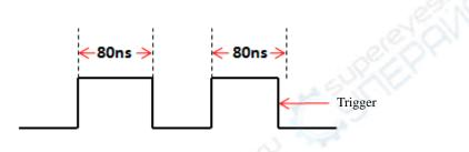
Figure 6-15 Trigger Time T<80ns
