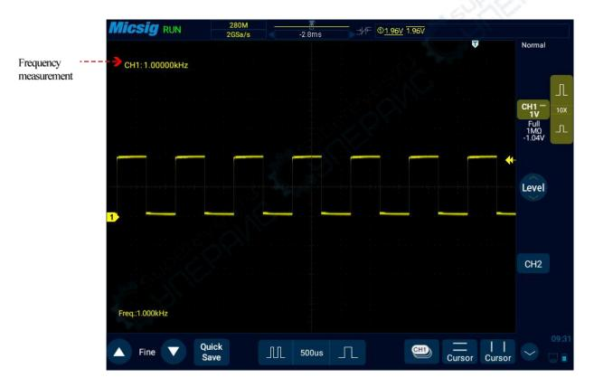
Figure 7-9 Frequency Meter Measurement
