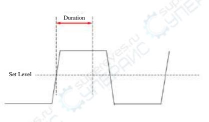
Figure 6-27 Timeout Trigger Schematics
