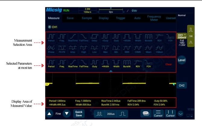
Figure 7-1 Automatic Measurement Menu
