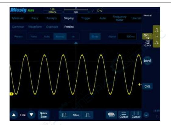
Figure 10-4 10MHz Sine Wave Variable Persist 500ms
