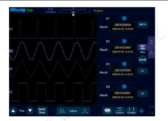
Figure 9-7 Restore Reference Waveform
