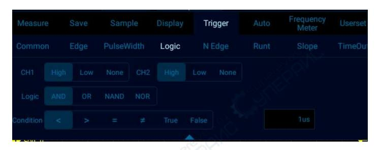
Figure 6-20 Logic Trigger Setting Menu
