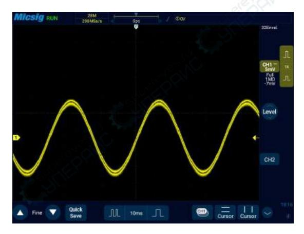
Figure 11-8 AM Signal in Envelope Sampling Mode (32)
