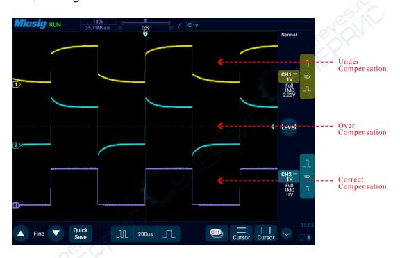
Figure 2-14 Probe Compensation
