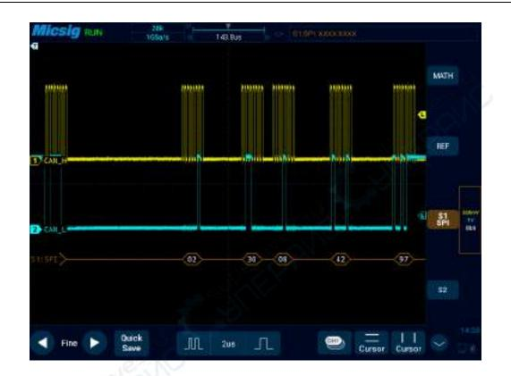
Figure 12-20 SPI Graphic Interface
