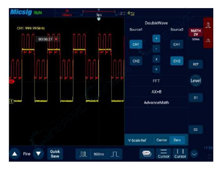
Figure 9-1 MATH Channel Waveform
