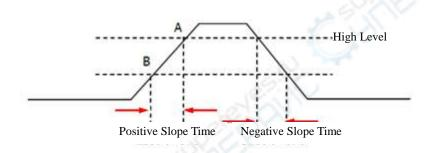
Figure 6-25 Positive/Negative Slope Time
