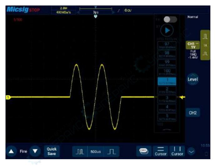
Figure 11-12 Single frame view of segmented storage
