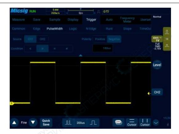
Figure 6-14 Negative Polarity Pulse Level Flip
