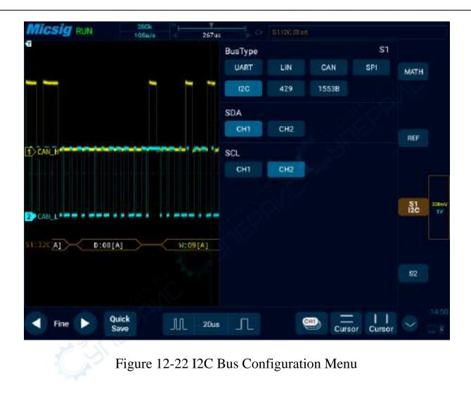
Notes: When SCL or SDA channel is set, the system will automatically set other channels.
