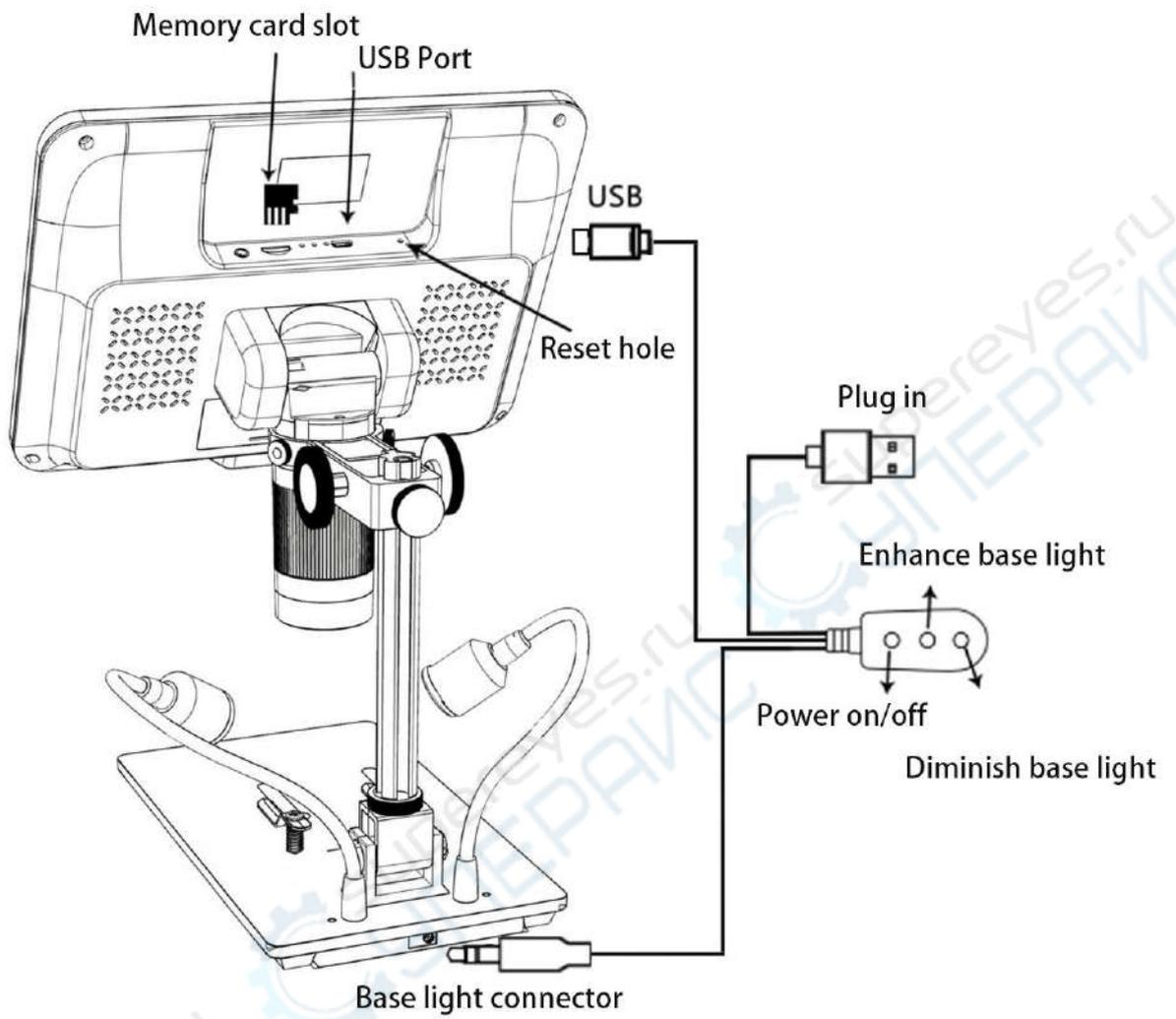
(Pic.5 Wiring Diagram)
