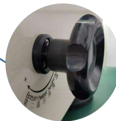
Bottom heater height adjustment. The distance between PCB and suction nozzle is 2-3mm.
