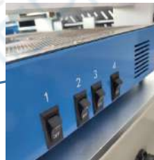
Infrared heating area control switch, 4 pcs, control 4 pcs heating plates in four corners, reduce the maximum power output, energy saving.
