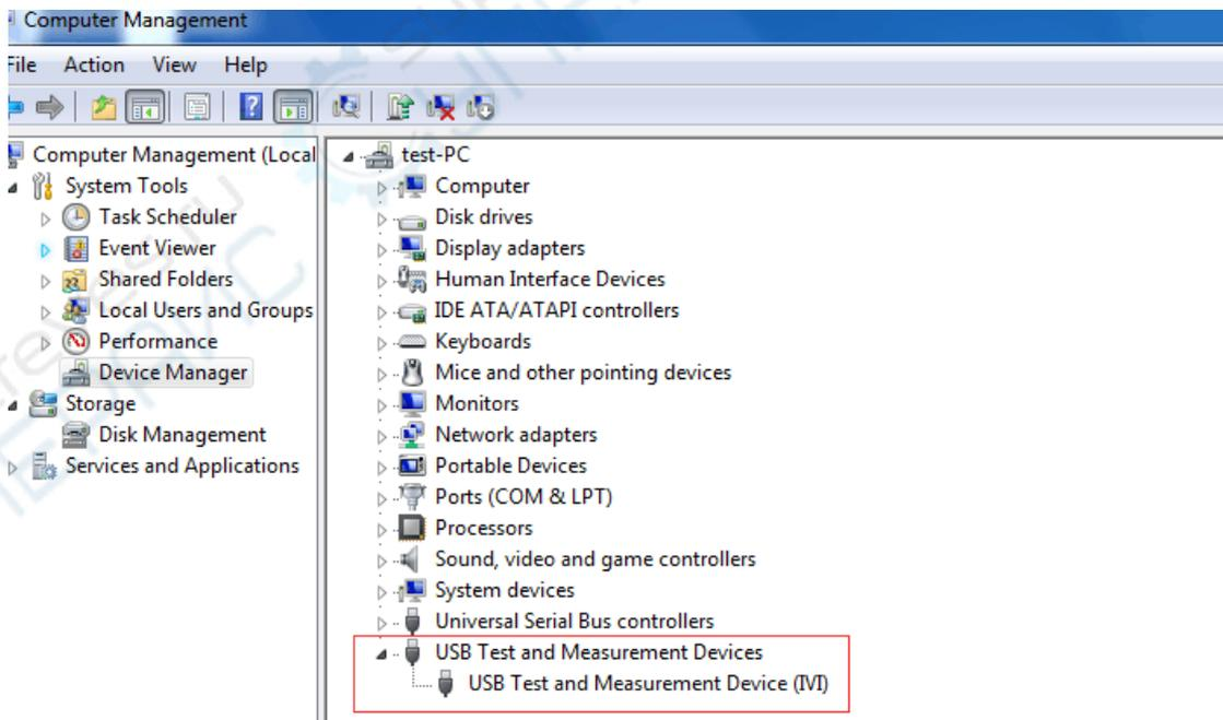
If "**USB Test and Measurement Devices (IVI)**" is displayed, that means the driver is installed successfully.
