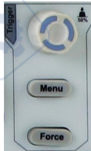
Figure 3- 13 Trigger Control Zone
