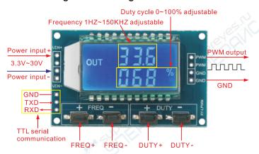
Output PWM amplitude=Input voltage
