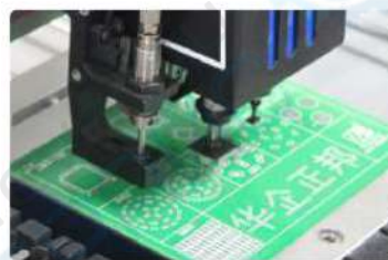
Double Mounting Head Working at the Same Time
