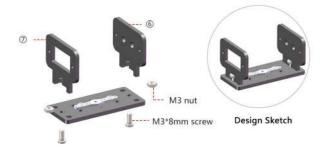
14 Assemble camera horizontal servo
