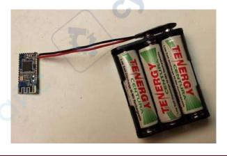
To protect the battery pack and module you should install the assembly in a case.
