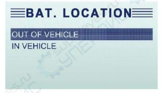
Scroll with the UP or DOWN button to highlight OUT OF VEHICLE or IN VEHICLE from BATTERY LOCATION menu and press ENTER to select the battery location.
