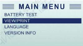
Review the test results on the screen. Use the UP or DOWN button to scroll back and forth through Battery Result, Charging Result and Cranking Result to view.
