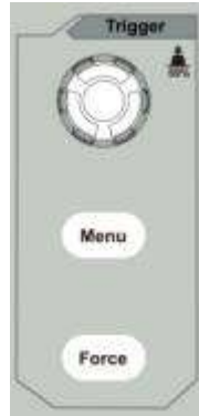
Figure 5-3: Trigger Control Area
