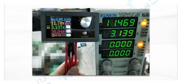
Note: The voltage display error is a normal phenomenon due to the voltage drop caused by the internal resistance of the wire.
