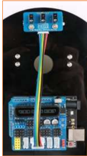
Figure 4.5.5 Infrared tracking module wiring physical map
