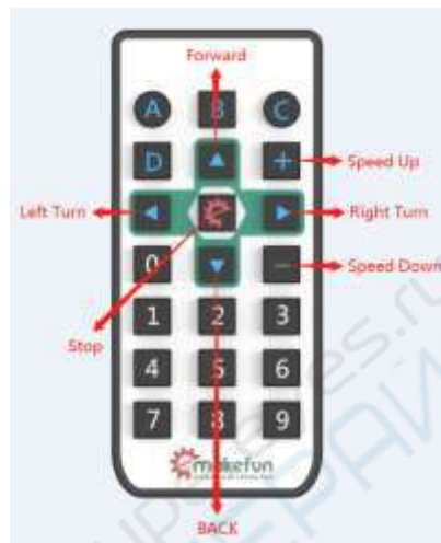
Figure 4.11.2 Infrared remote control button function definition
