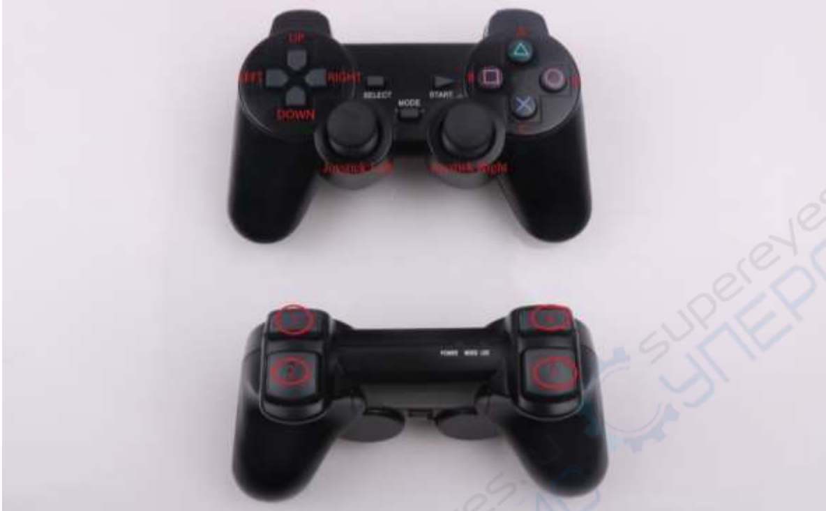
Figure 4.15.2 PS2 handle function button diagram
