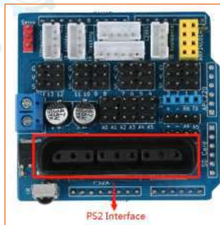
Figure 4.14.3 PS2 handle connection diagram
