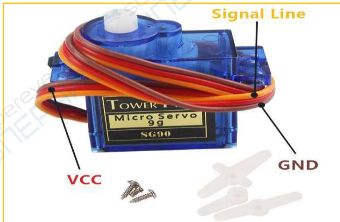
Figure 4.7.2 SG90 servo machine physical map
