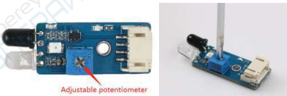
Figure 4.2.2 Schematic diagram of detection distance adjustment
