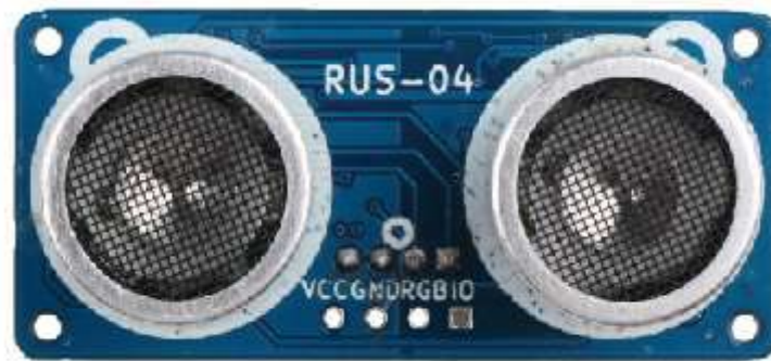
Figure 4.8.1 Physical diagram of the ultrasonic module
