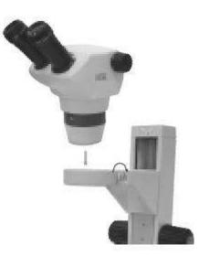
Warning: Do not tighten the screw too tight as this will make damage to the instrument.
