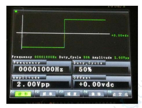
The function description of the button in this interface: Button F1: Select the type of waveform
