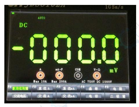
The function description of the button in this interface: Button F1: Select DC or AC voltage Button F2: Select DC or AC current (A) Button F3: Select DC or AC current (mA) Button F4: Select on or off or capacitor Button F5: Select resistor or diode
