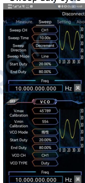
Figure 3-9-37 Voltage control duty cycle
