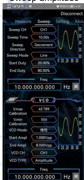
Figure 3-9-36 Voltage control amplitude
