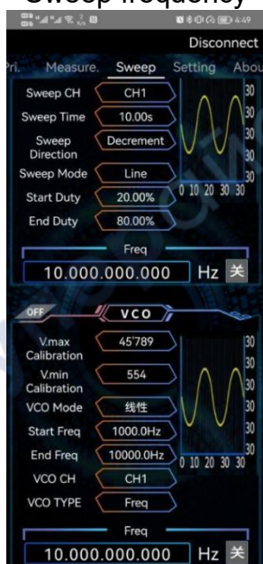
Figure 3-9-35 Voltage control frequency
