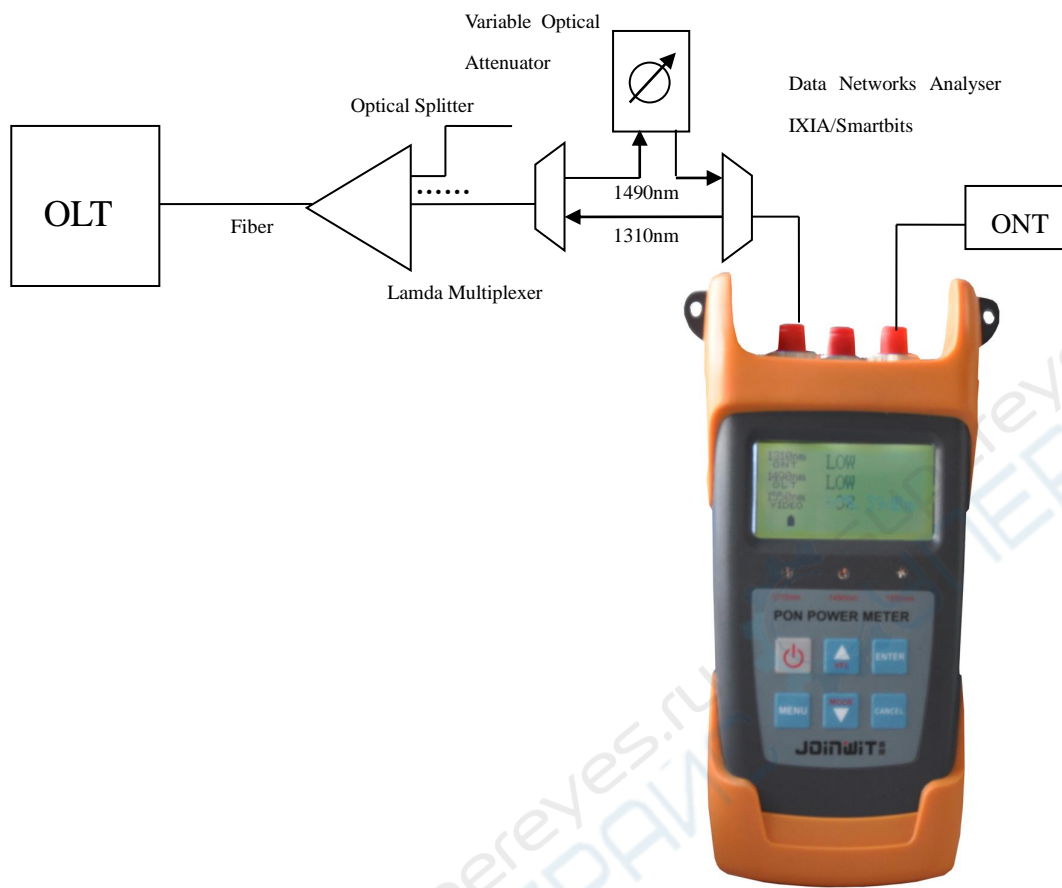
ONT The sensitivity test configuration diagram
