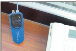
Connect launcher and LAN cable port to be traced in right way
