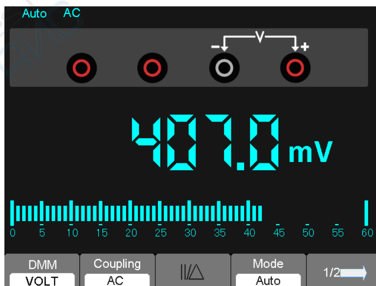
Figure 7-7 AC voltage Measurement
