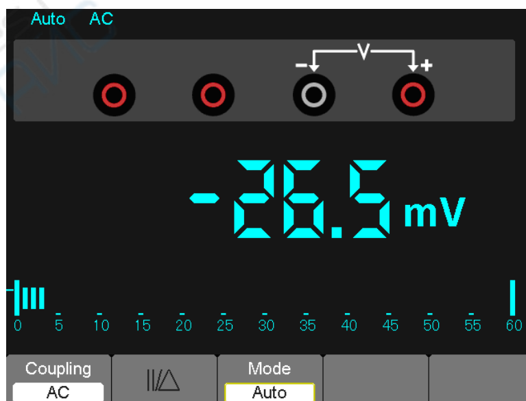
Figure 7-7 AC voltage Measurement
