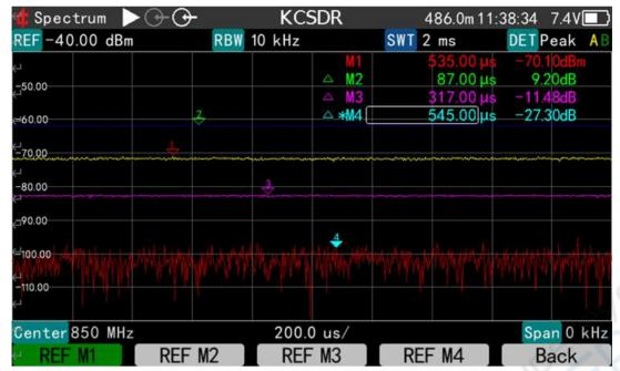
To receiver, this function is meant to switch to receiver mode, and set the marker frequency as the receiving frequency. With auto-peaking function enabled, the marker would stick to the peak spectrum line instantaneously.
