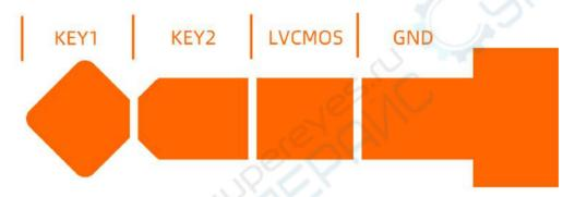
KEY1 and KEY2 are used to connect the telegraph key. While using a manual key it should connect to KEY1 and GND. To use an automatic key user should connect KEY1, KEY2 and GND. The driving voltage for key is usually 1.8V.
