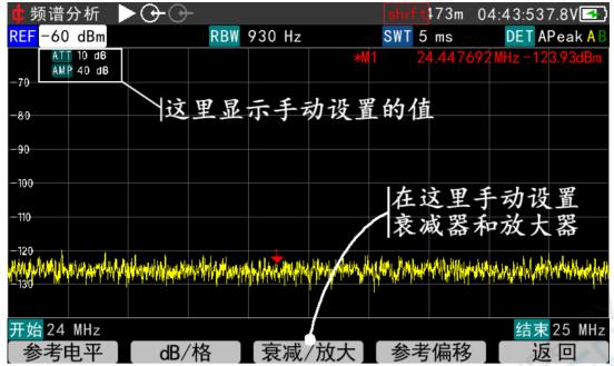
Likewise, switching AMP off or increasing ATT value cannot reduce the interactive interference within the machine, yet it might even become unneglectable without the amplifer's noise.
