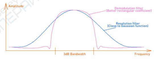
For wide-band signals, the wider the resolution bandwidth or demodulation bandwidth is set, the larger the readout will be.
