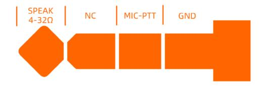
Those common hand speaker mic compliant to this pin definition can be used. When using normal Condenser or Dynamic microphone, Connect the microphone to MIC-PTT and GND then KC908 considered the PTT is pressed. The sensitivity of microphone is about 50mV. The speaker should be connected to the SPEAK and GND pin. When using headphone user should turn down the volume before plugging. In KC908's FUNC menu user can set turn off or not the built-in speakers after plugging in this port.
