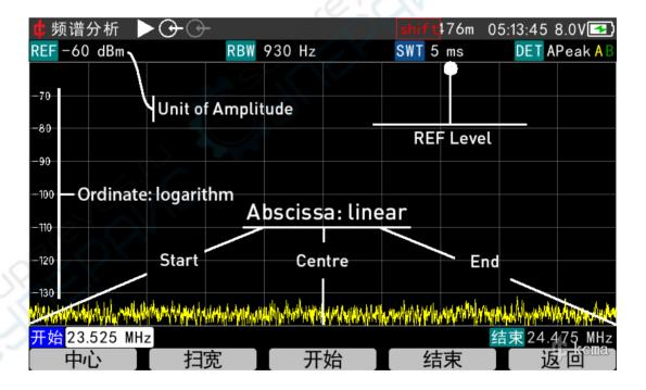
The horizontal coordinates of KC908 are on a linear scale. If the leftmost coordinate represents 0Hz, and the rightmost coordinate represents 10GHz, then the center is 5GHz, because people are more concerned about the center frequency, so the center frequency (CENT, CF) and sweep width (frequency span,SPAN) are often used to set the instrument.
