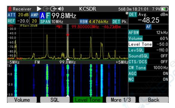
Pic: In searching-on-foot scenario, setting the central point on the current reading level would be helpful to hear the change.
