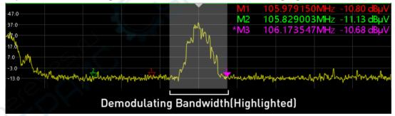
In MODU menu, DETECTOR defines the way level meter detects the signals. This setting can be neglected if the user just want to take a glance of the level/field strength. Whereas a precise field strength measurement demands the DETECTOR parameter properly set accroding to different modulating methods of the signal, or accroding to relevant standards.
