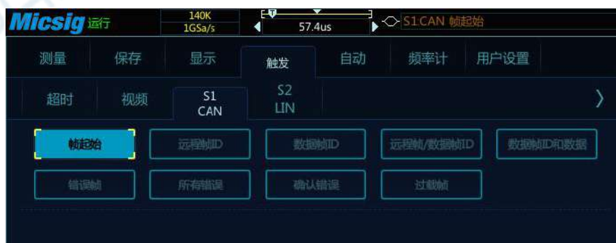
图12-14 CAN 触发方式配置菜单
