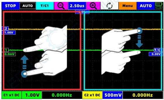
In the red area in the figure, slide up and down with a single finger, and the operability icon is C1, C2, V1
