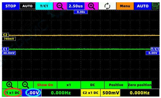
In this interface, you can zoom in and out the waveform voltage range of C1,
