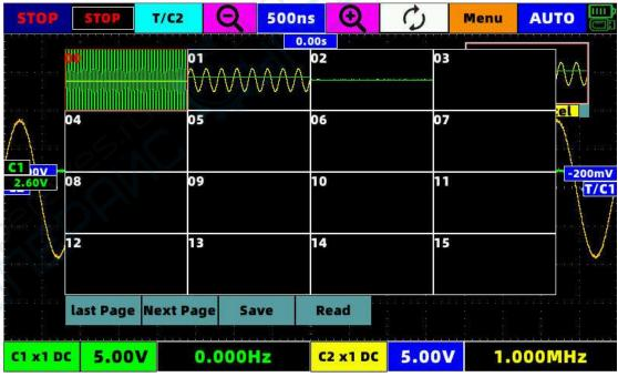
After clicking to store the waveform, the current waveform will automatically stop and enter the stop state.
