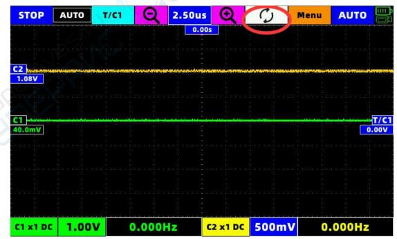
This switch key can switch between oscilloscope and signal generator with one key.
