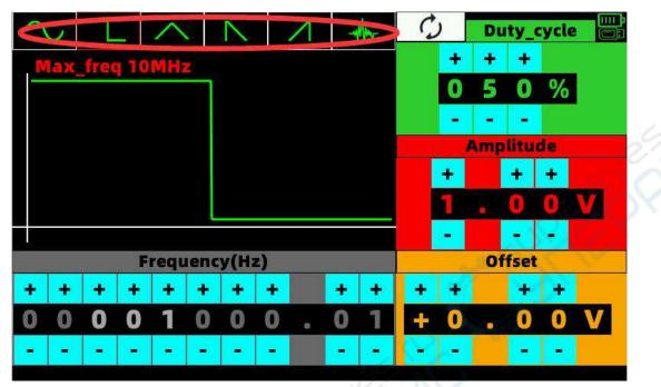
Through the corresponding +,- to modify the frequency, amplitude, offset, duty cycle and other signals, the waveform will be directly changed in real time. The red circle area can select the waveform to be output.
