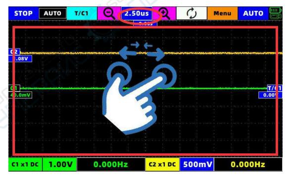
(Horizontal) Two-point touch the time base of the waveform can be changed (the value in the red circle in the figure)
