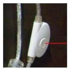
Push the button of the dimmer that located on the USB cable to freeze an image.
