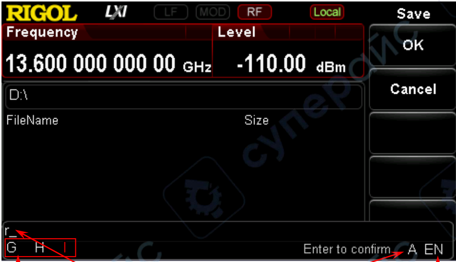
Letter Selection Area Letters Entered Uppercase/Lowercase English Input Mode (a) English Input Mode
