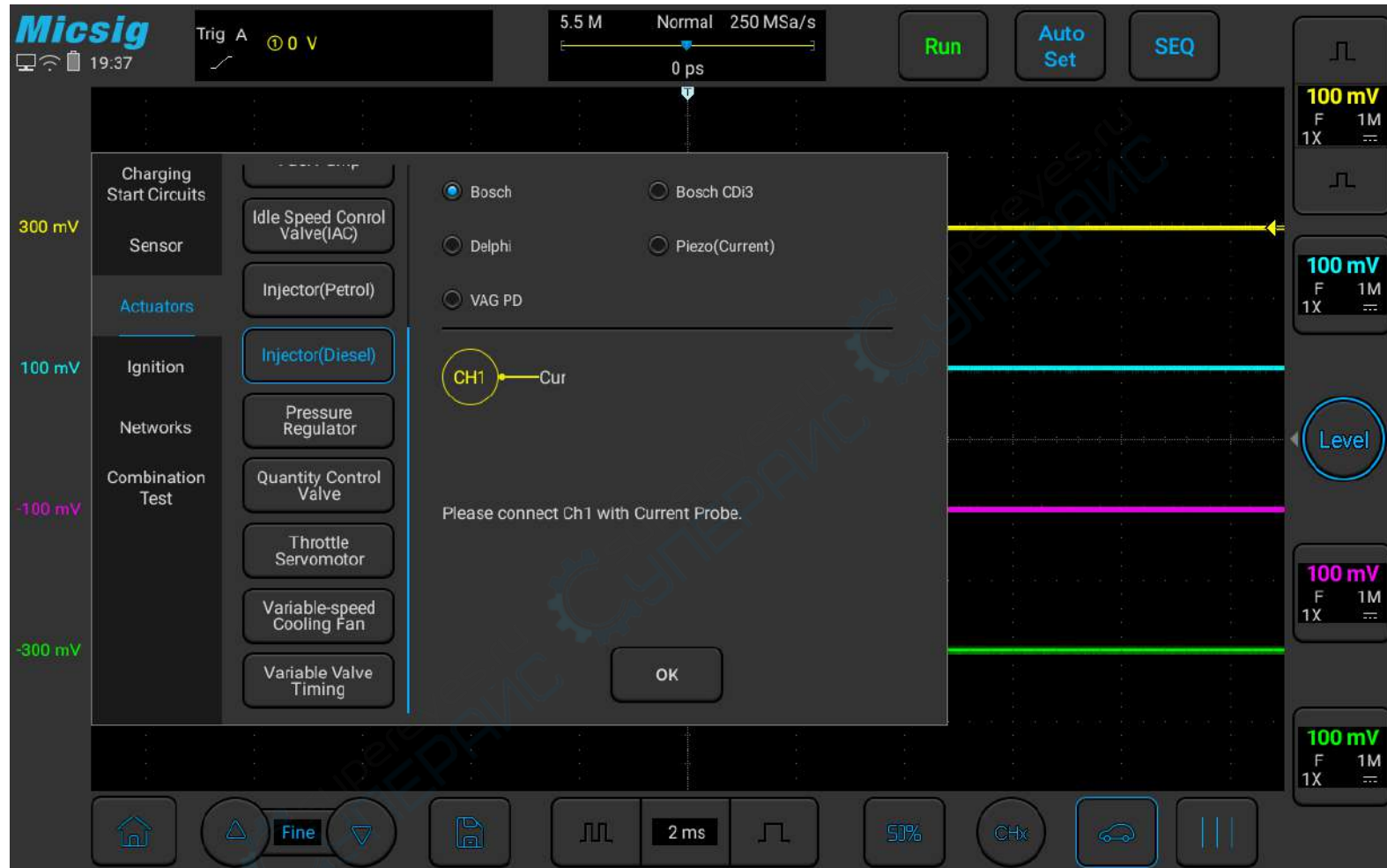
Figure 3-33 injector (diesel engine) test
