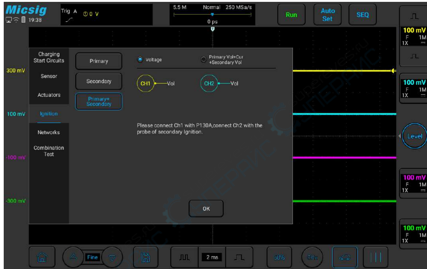
Figure 3-43: Primary + Secondary ignition test
