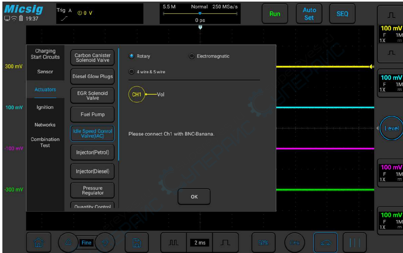
Figure 3-31 Idle speed control valve test
