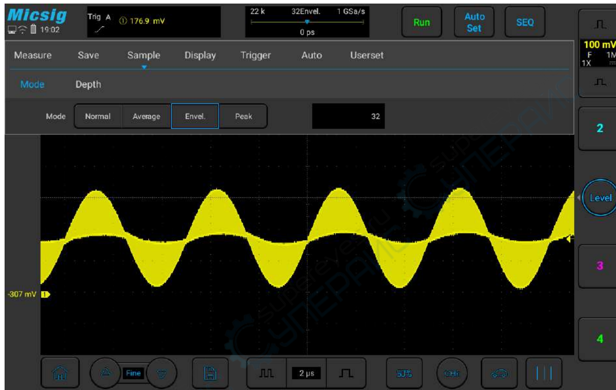
Figure 11-8 AM Signal in Envelope Sampling Mode (32)
