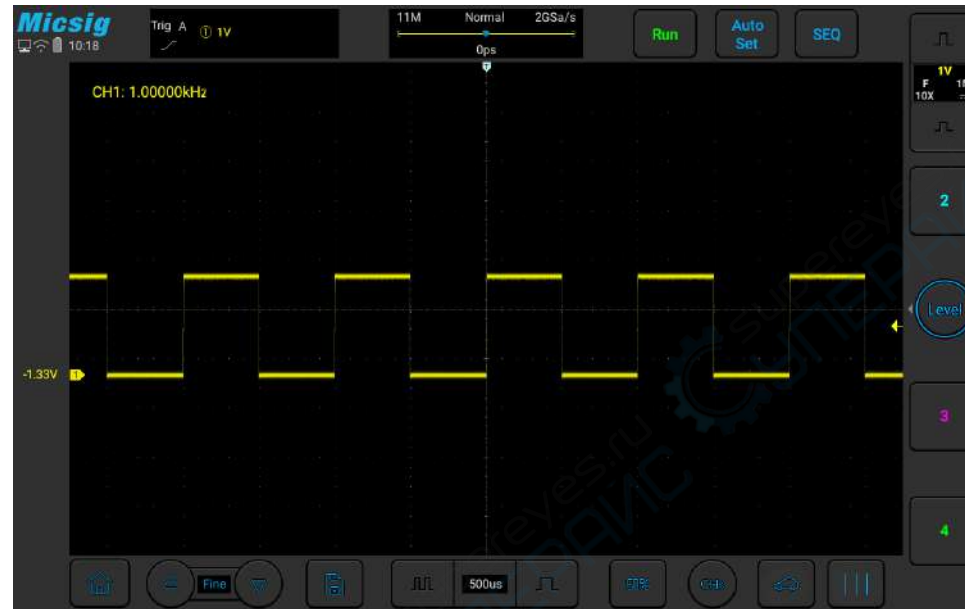
Figure 7-10 Frequency Meter Measurement
