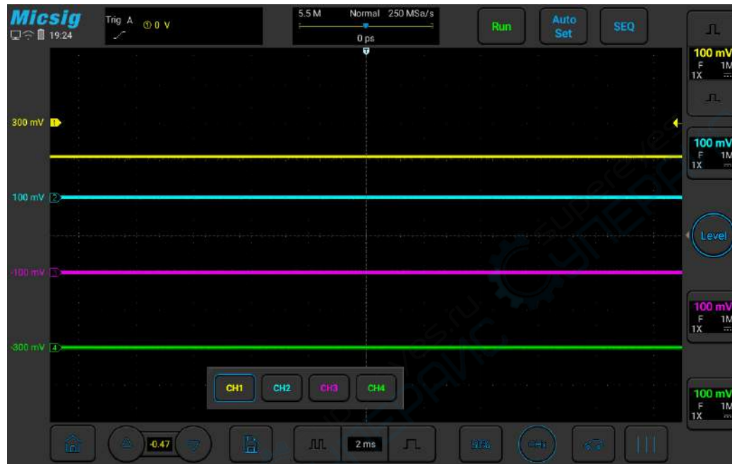
Figure 2-13 Manual zero calibration
