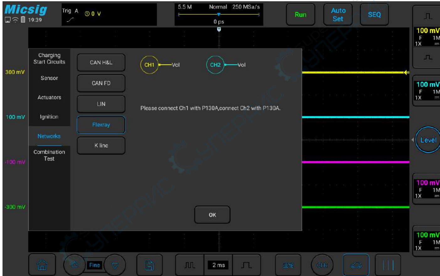
Figure 3-48: FlexRay bus test
