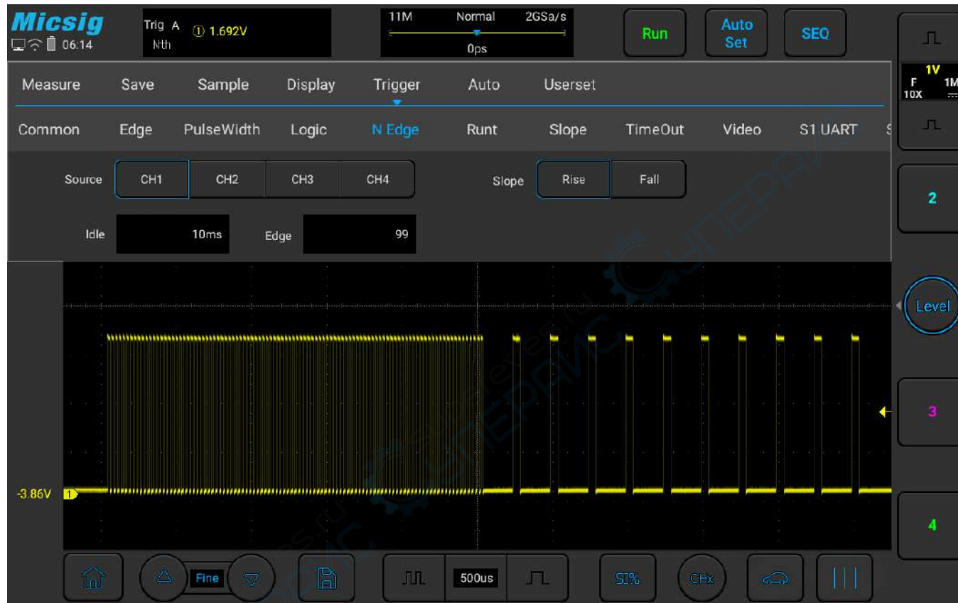
Figure 6-23 Nth Edge Trigger Menu
