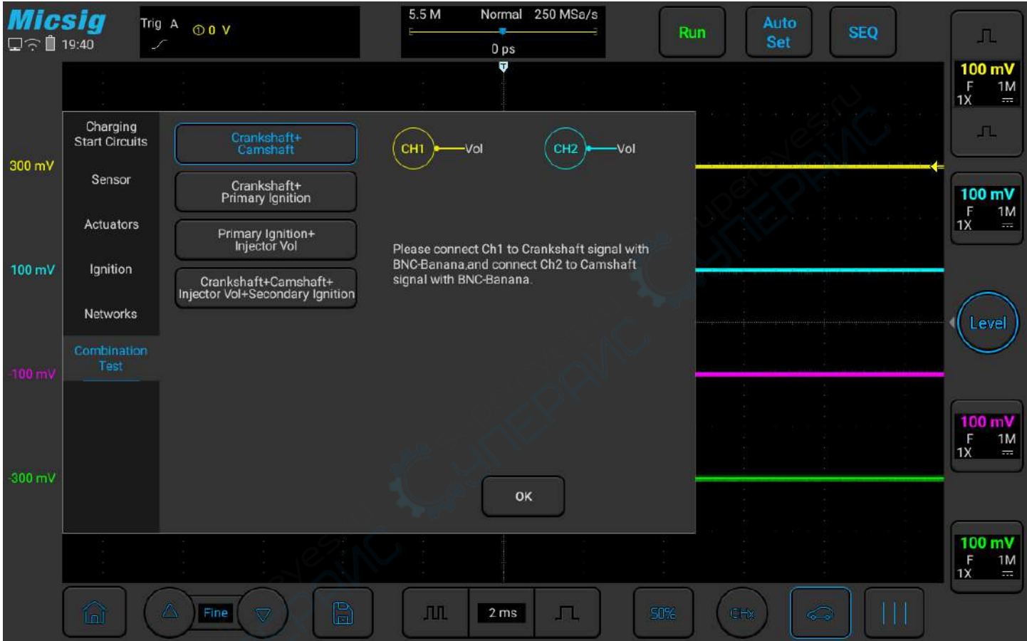
Figure 3-50 Crankshaft + Camshaft Combination Test
