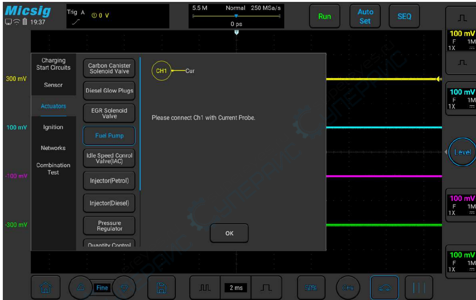
Figure 3-30 Electronic fuel pump test
