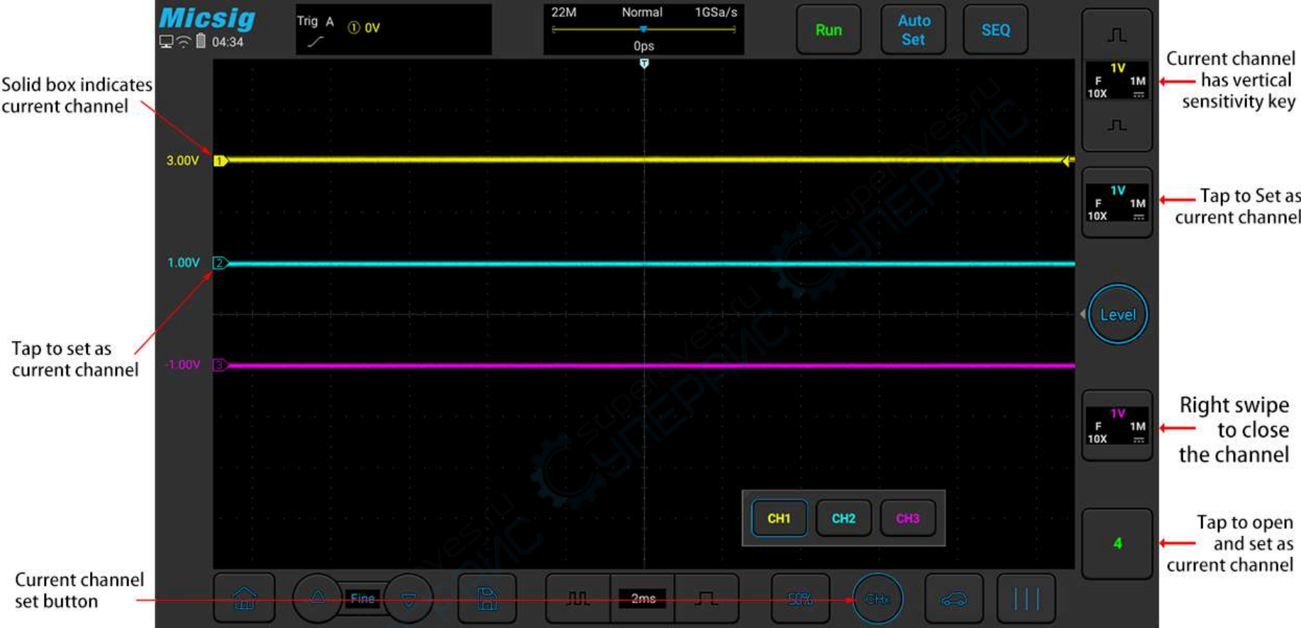
Figure 5-4 Channel Open, Close and Switching
