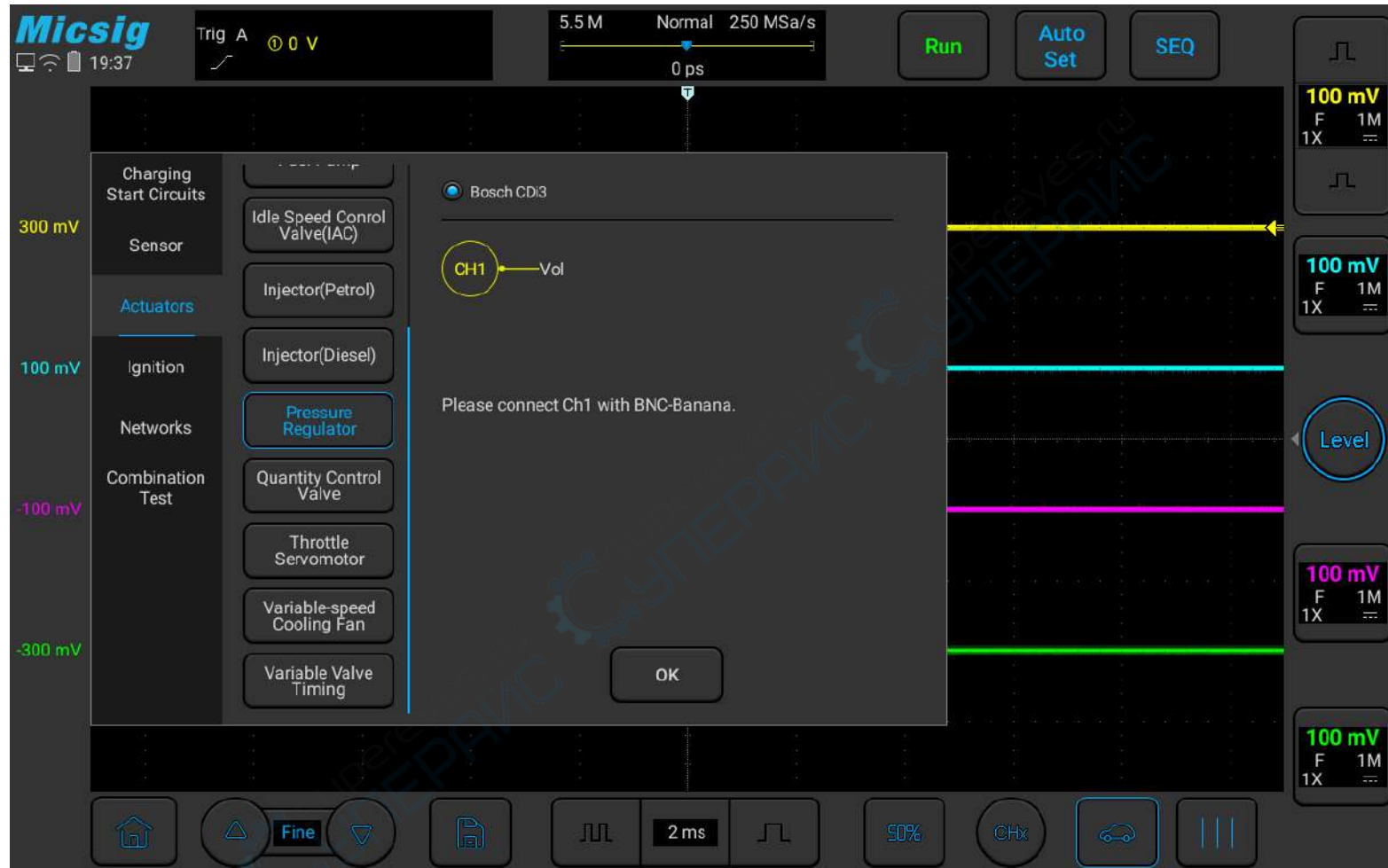
Figure 3-34 Pressure Regulator test
