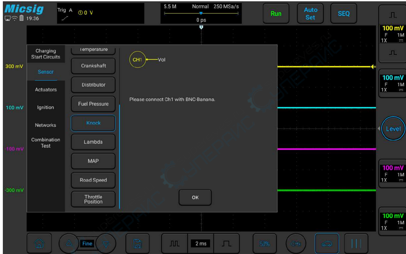
Figure 3-19 Knock Sensor test
