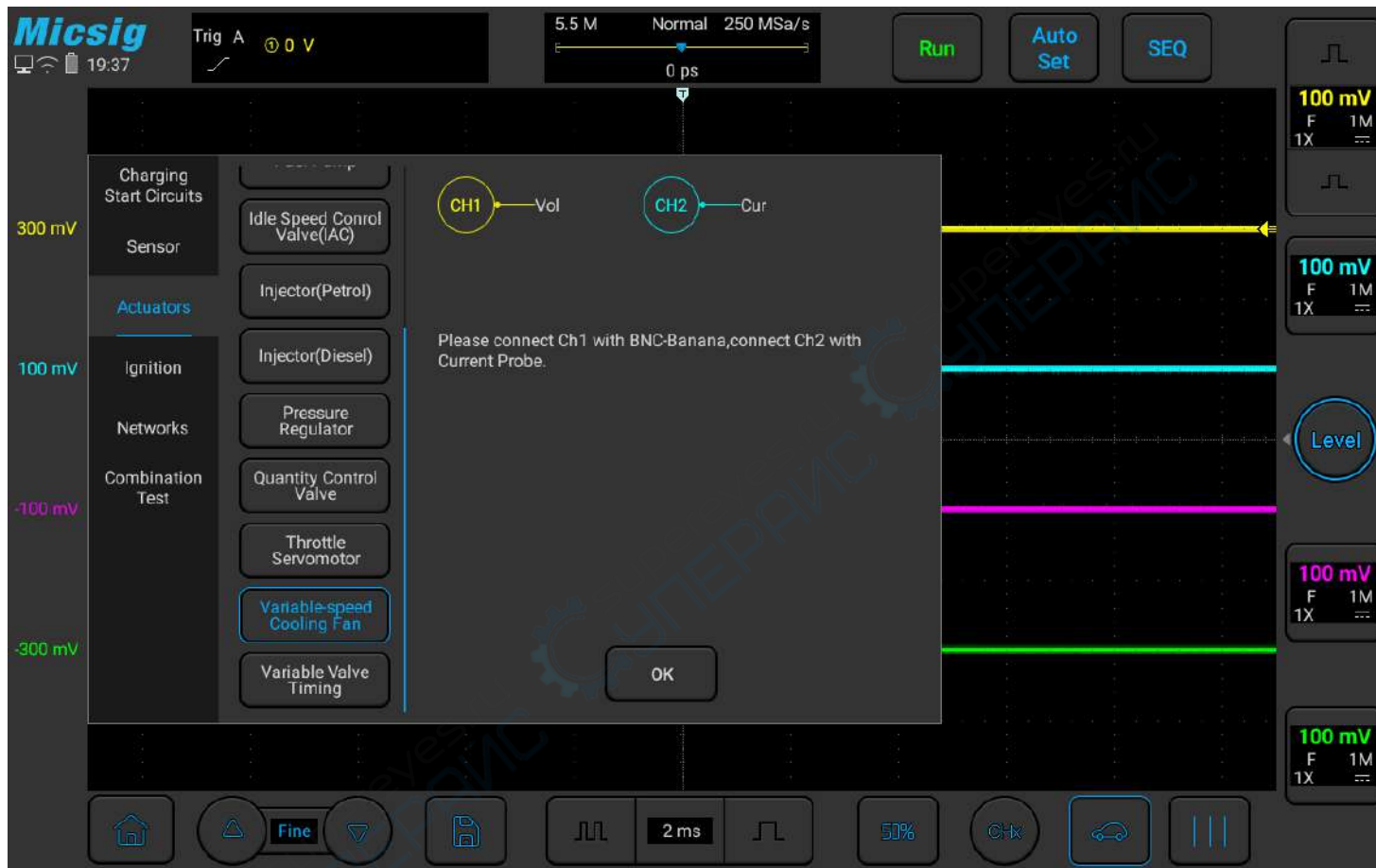
Figure 3-37 Variable-speed Cooling fan test
