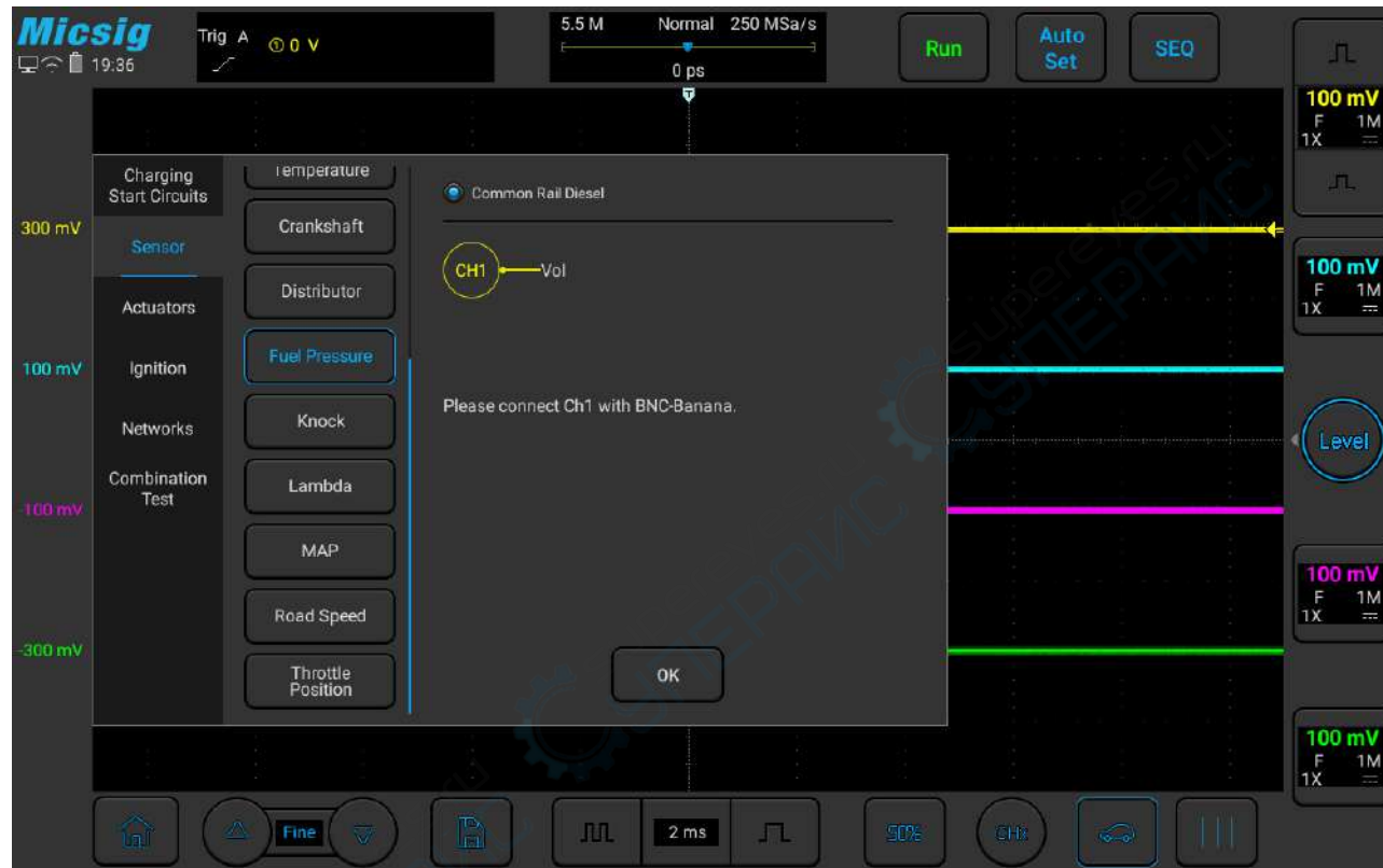
Figure 3-18 Fuel Pressure Sensor Test
