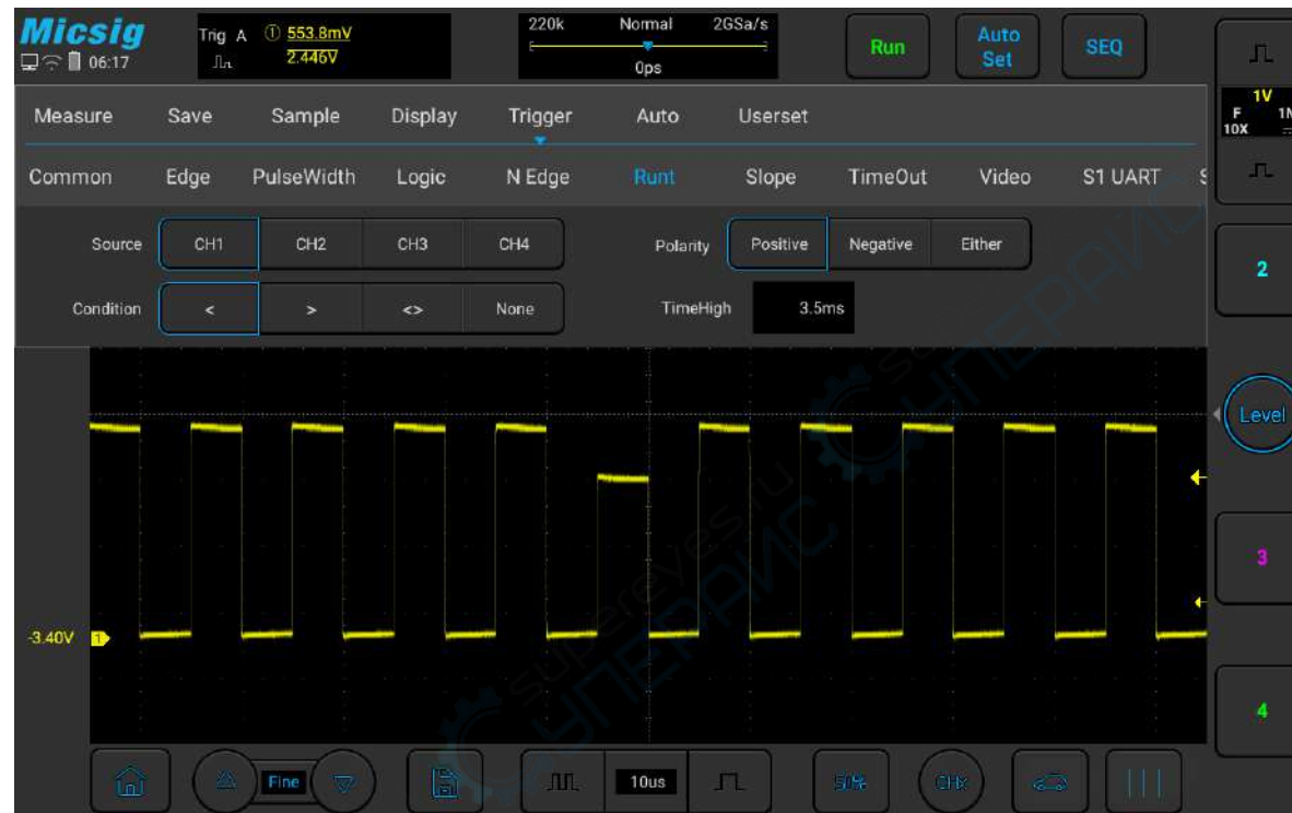
Figure 6-25 Runt Trigger Setting Menu
