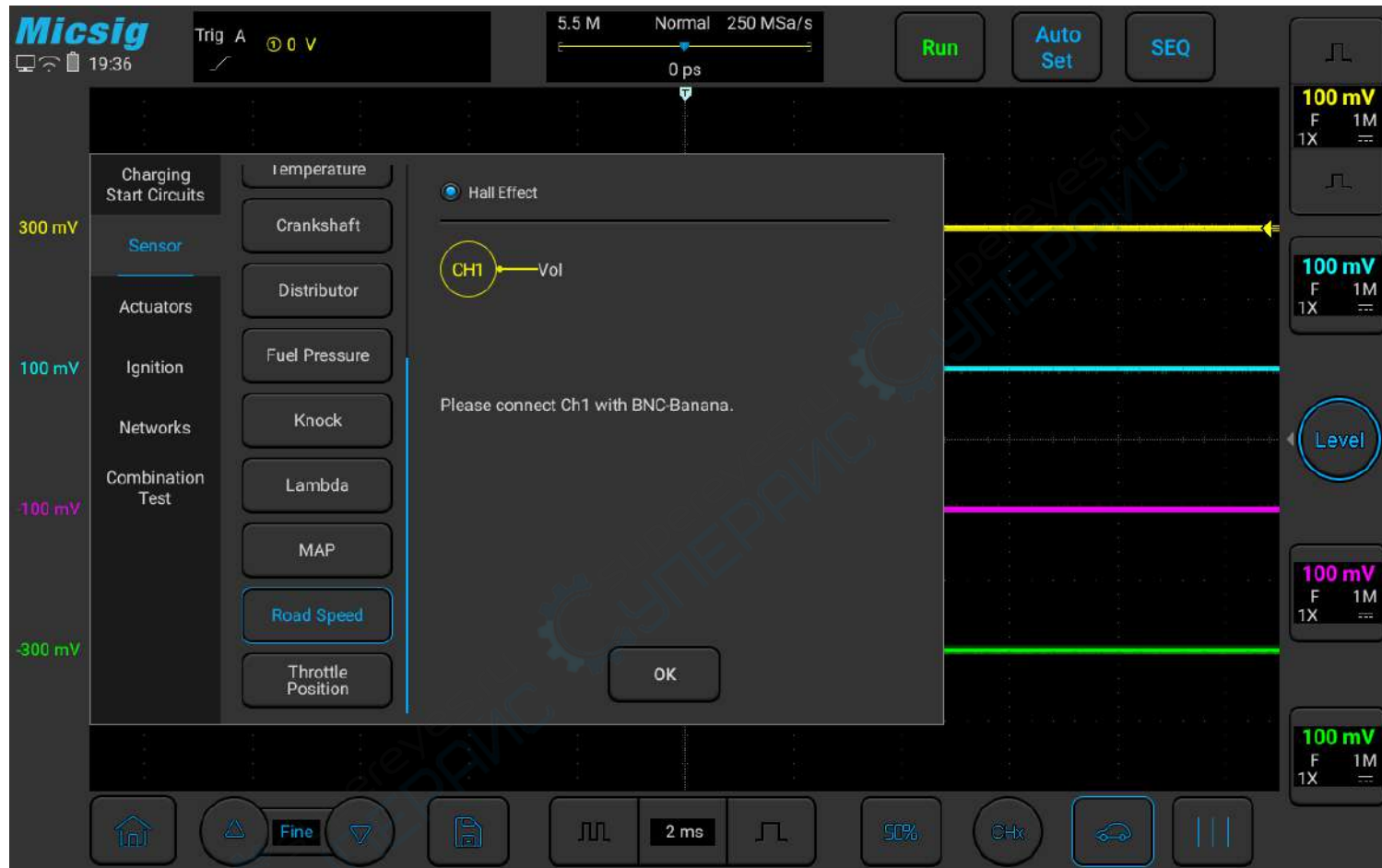
Figure 3-23 Vehicle speed sensor test
