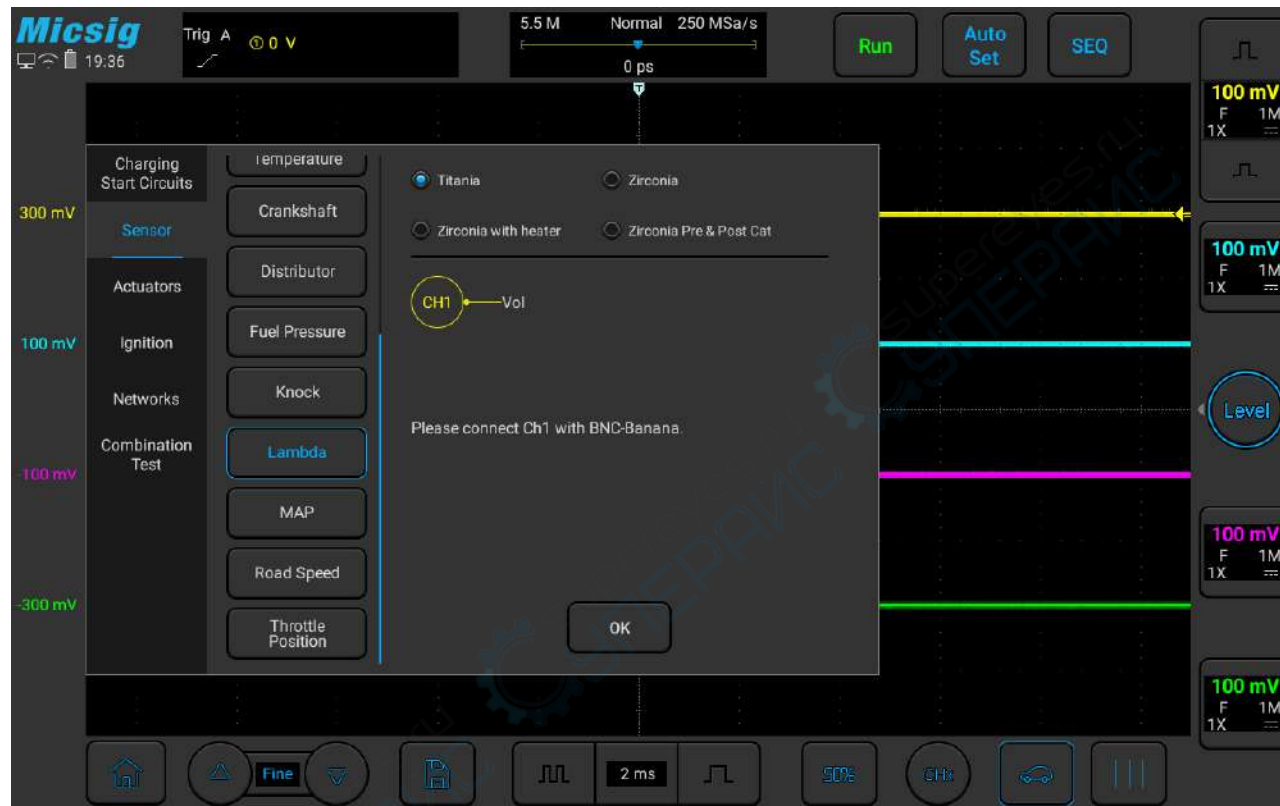
Figure 3-20 Lambda (oxygen sensor) test
