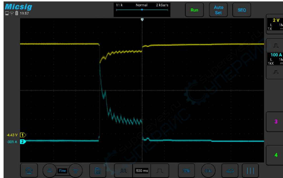
Figure 3-7 Starting voltage and current
