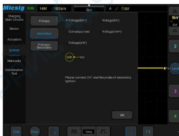
▲ The ignition system of a car is usually composed of primary and secondary coils and spark plugs. Can test both Primary and Secondary ignition signals, to find out possible malfunction.
