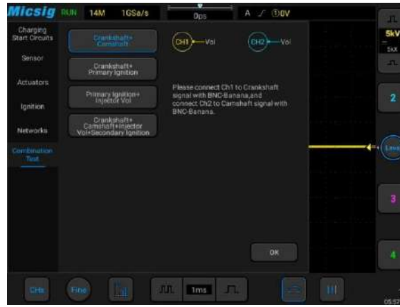
▲ The ignition system of a car is usually composed of primary and secondary coils and spark plugs. Can test both Primary and Secondary ignition signals, to find out possible malfunction.
