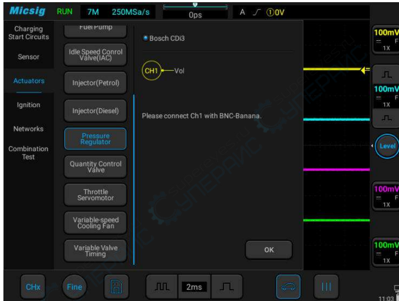
Figure 3-34 Pressure Regulator test
