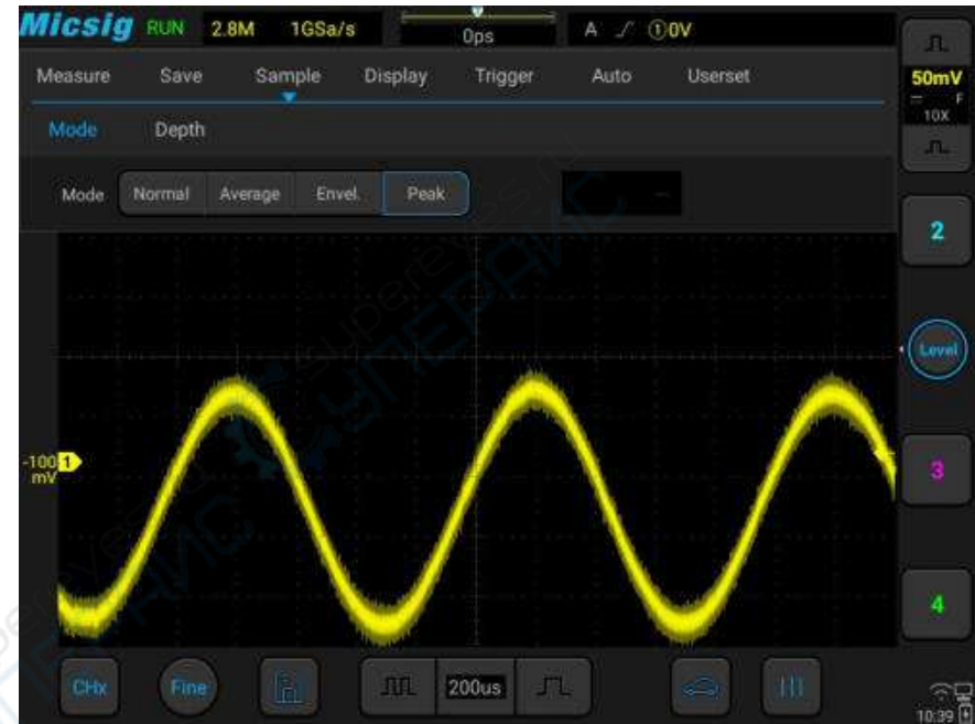
Figure 12-6 Sine Wave with Burr Peak Sampling Mode
