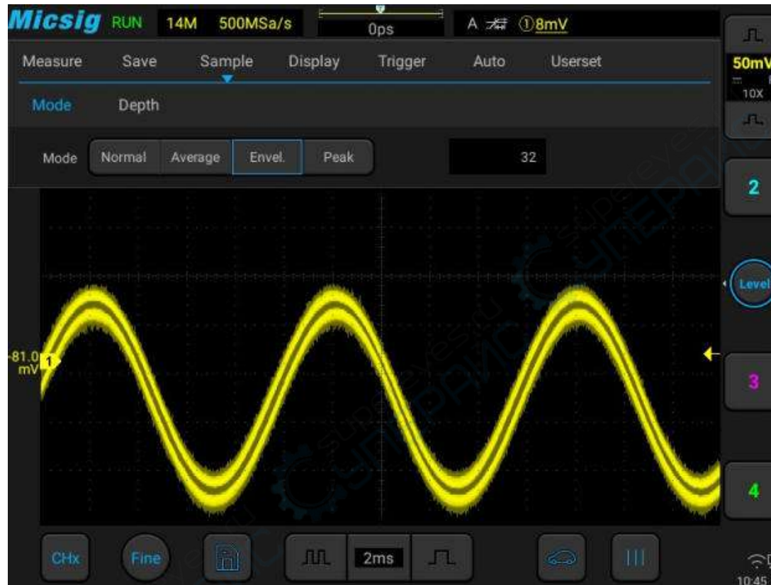
Figure 12-8 AM Signal in Envelope Sampling Mode (32)
