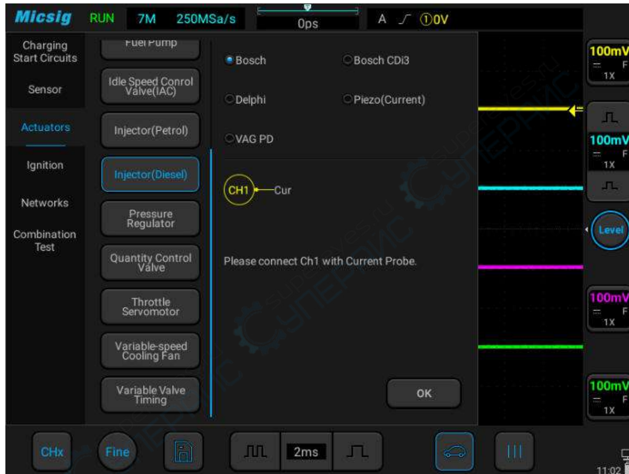
Figure 3-33 injector (diesel engine) test
