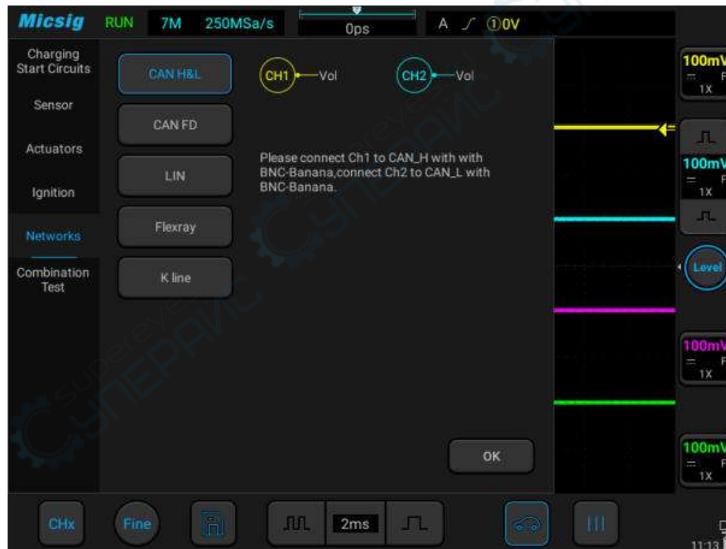
Figure 3-45 CAN BUS Test
