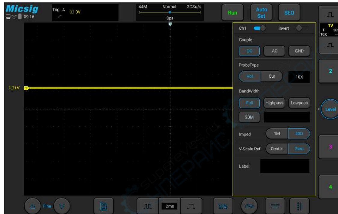
Figure 4-17 Channel Input impedance
