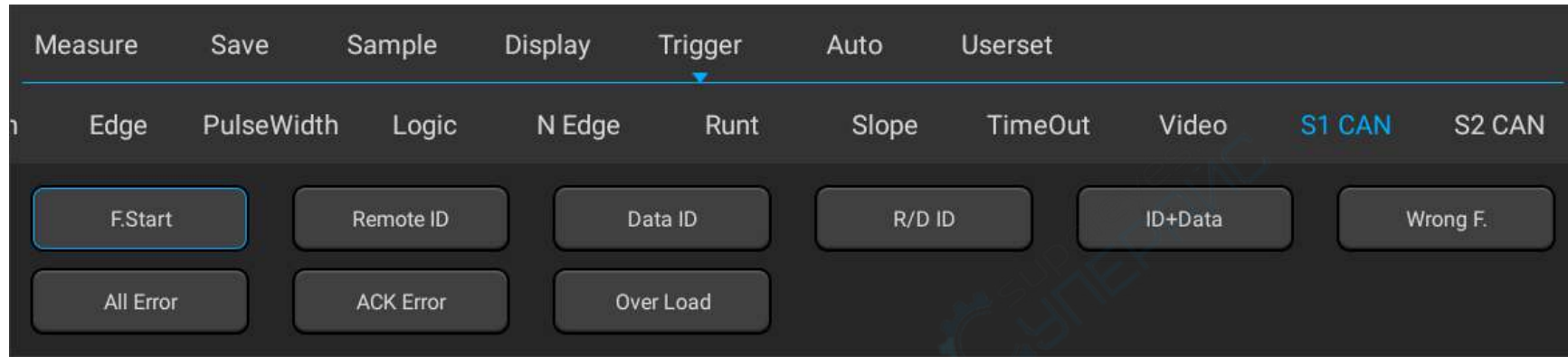
Figure 11-15 CAN Trigger Mode Configuration Menu
