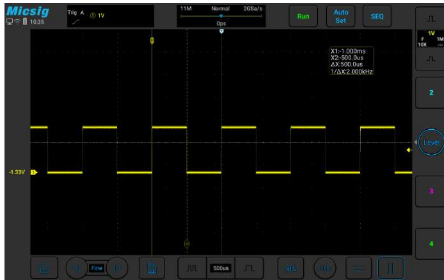
Figure 6-13 Cursor Measurement Pulse Width
