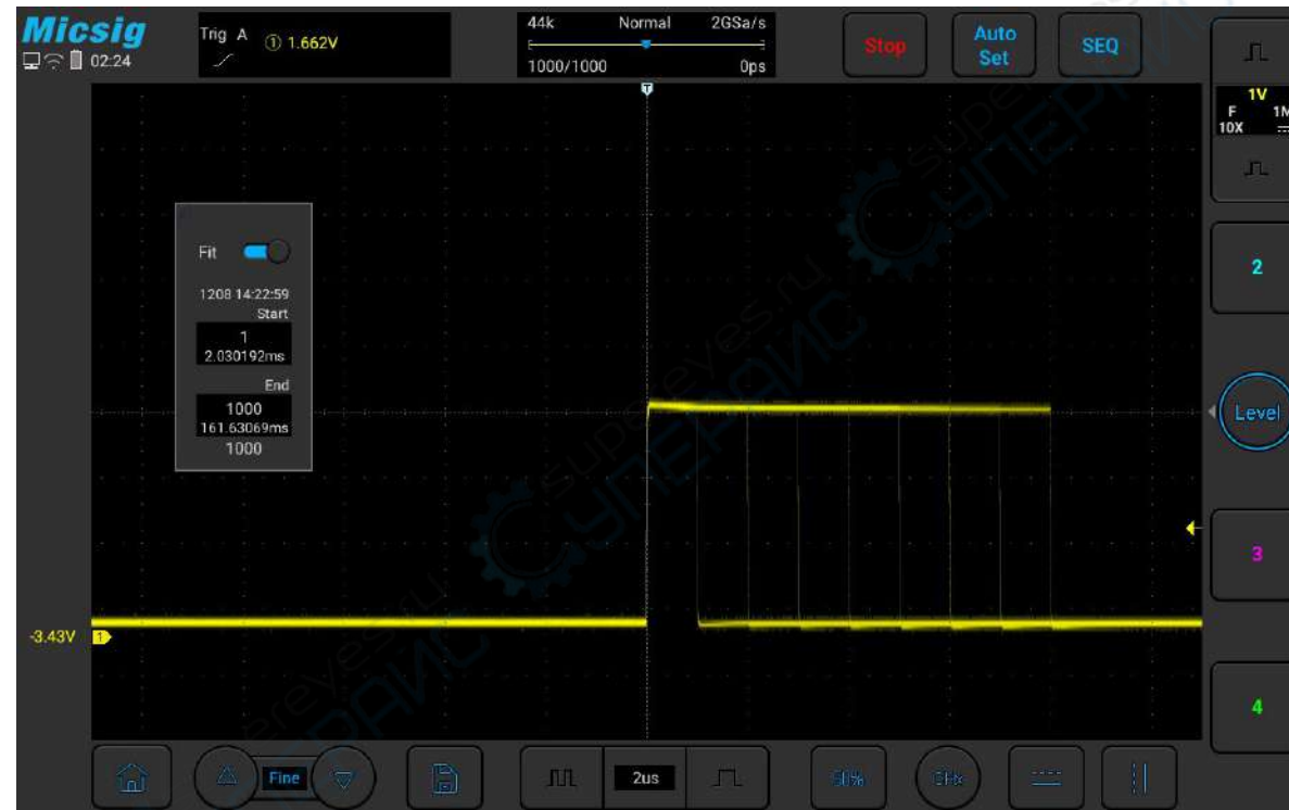
Figure 10-13 Segmented storage fitting view
