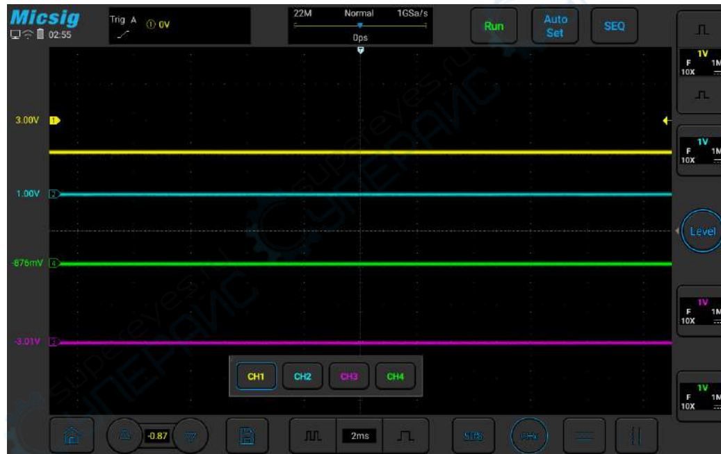
Figure 2-13 Manual zero calibration
