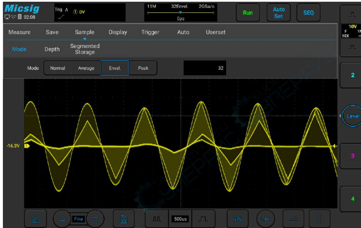
Figure 10-8 AM Signal in Envelope Sampling Mode (32)
