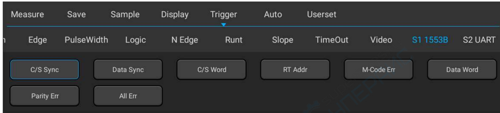
Figure 11-31 1553B Trigger Mode Configuration Menu
