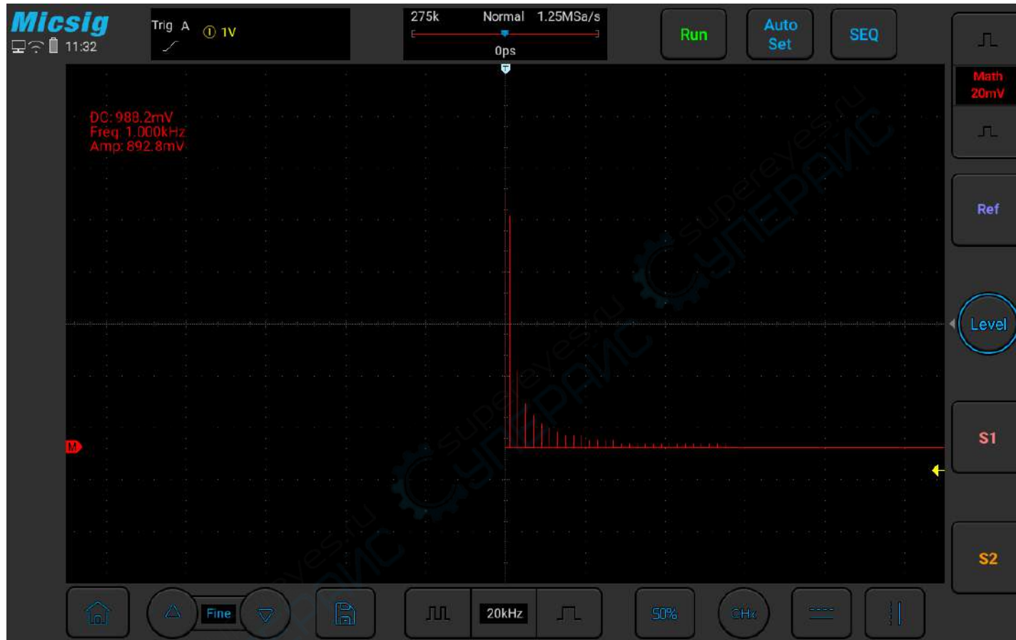
Figure 8-4 Spectrum Amplitude as V-Hz
