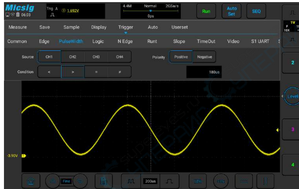
Figure 5-14 Pulse Width Trigger Setting Menu
