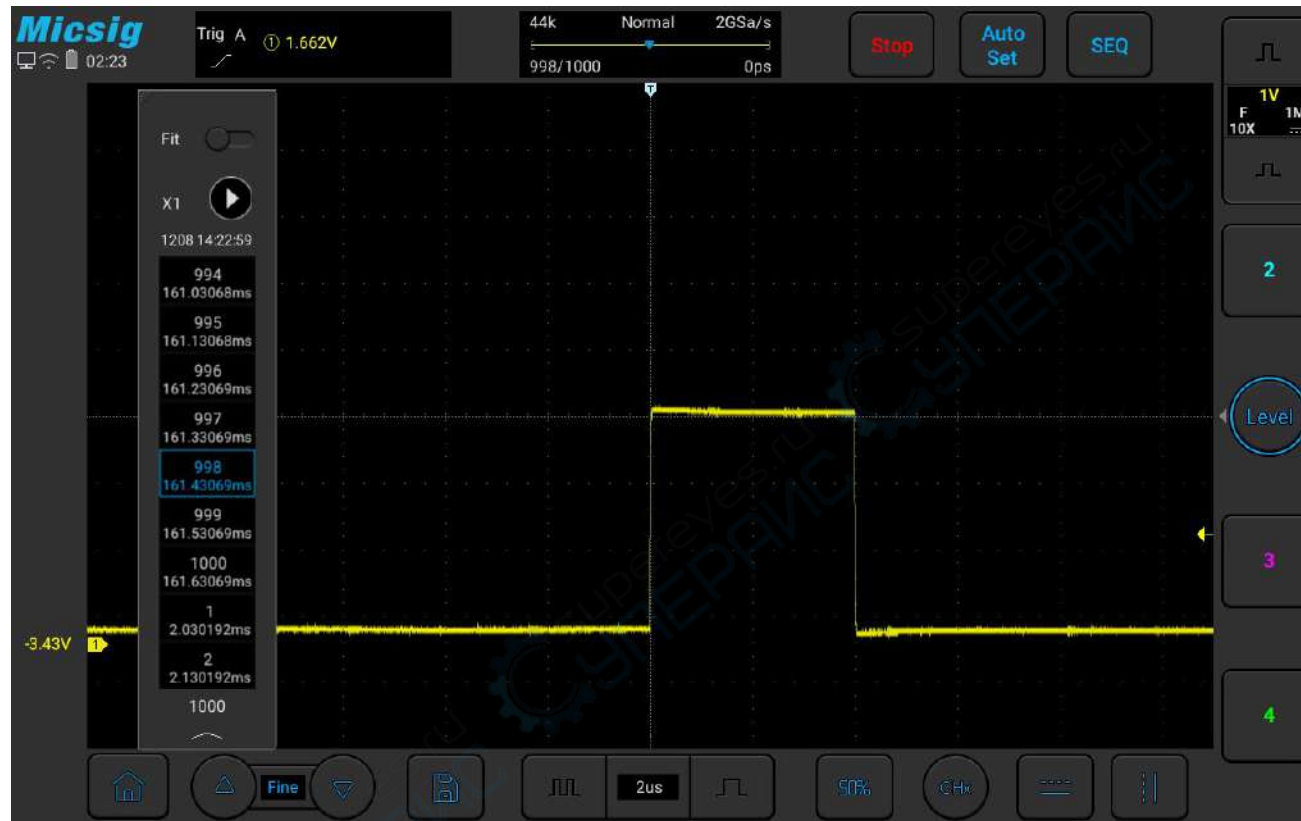
Figure 10-12 Single frame view of segmented storage
