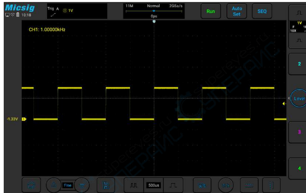
Figure 6-10 Frequency Meter Measurement
