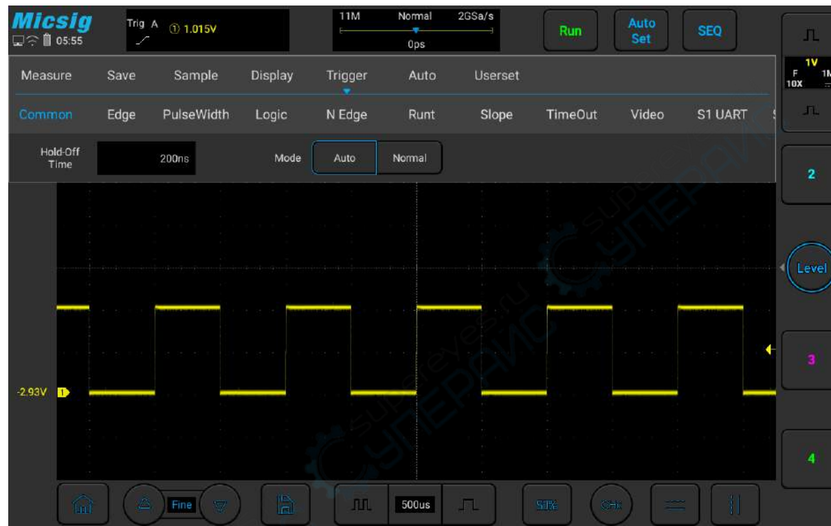
Figure 5-5 Oscilloscope Trigger Mode Setting
